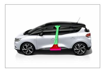
Figure 27 – Illustration of a B-pillar
