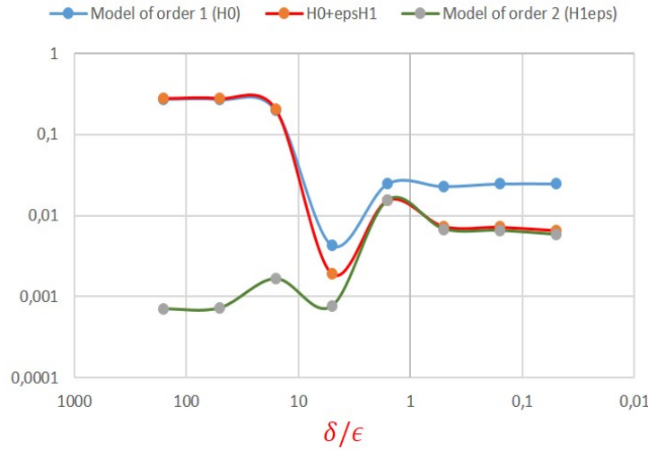
Figure 3.13: Relative L^2 errors of the solutions H_0 and H_\epsilon^1 of the equivalent models of order 1 and 2 versus the parameter \tilde{\sigma} for \epsilon = 4\text{cm}
