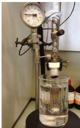
**Figure III. 17** Reactor used for etherification of glycerol with *tert*-butyl alcohol reaction.
