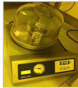
Figure 3-20: vacuum chamber used for filling the liquid in the micromachine by sucking air from the chamber.
