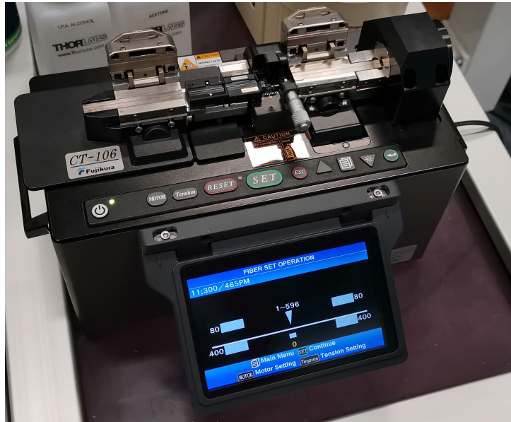
Figure 5.3: Automated optical fiber cleaver Fujikura CT-106 with variable tension.
