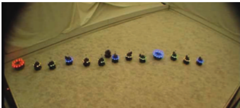
Figure 2.1: Example of collective chain formation. From [Nouyan et al., 2009], reproduced with permission ©2009 IEEE.
