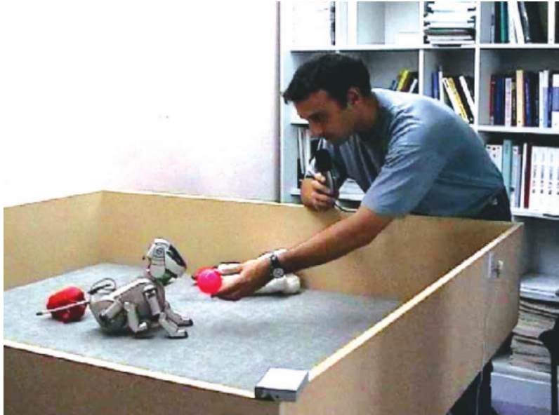
Figure 3.2: Example of the AIBO game dialog between robot and a human. The robot performs image segmentation and tries to associate words spoken to the human (i.e. “ball”) to the actual ball. For the interaction to be successful, the robot first has to be put in the right conditions by specific keywords. Reproduced from [Steels, 2001] ©2001 IEEE.
