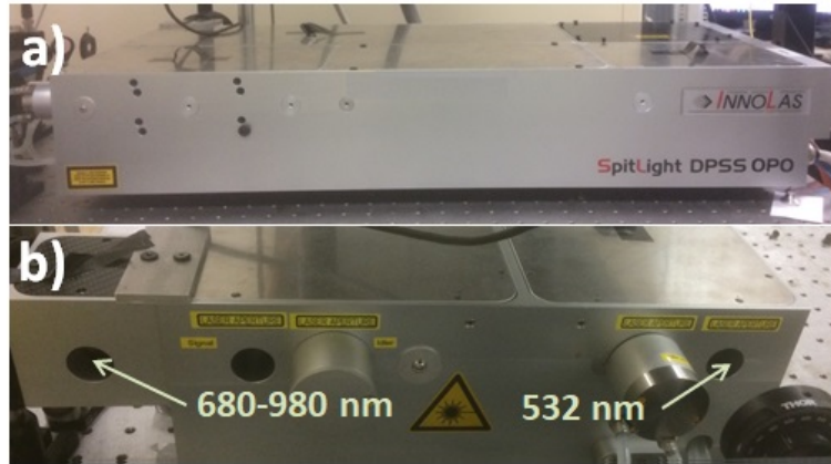
Fig. 2.2 (a) The laser head unit (side view). (b) The front view of the laser, with the output windows for 532 nm and 680-980 nm .
