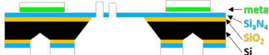
Figure 3.2. Cross-sectional view of the Si wafer during the different fabrication process steps. (a) The membrane and cleave lines are defined by laser lithography into a photoresist on the backside of the wafer. (b) The \text{Si}_3\text{N}_4 and \text{SiO}_2 layers are etched through the opened windows in the photoresist using RIE. (c) If slits in the membranes are desired: a laser lithography on the front side is carried out, (d) followed again by the same RIE steps. (e) The wafer is then immersed in a KOH bath which etches the Si. (f) In the last step a laser lithography is carried out on the front side of the wafer defining the metal contacts and any desired markers or labels. (g) The metal is then deposited and (h) lifted off.
