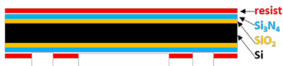
(b) RIE on back side defining membrane and cleave lines
