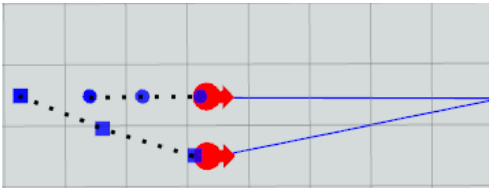
Figure 5-11: Behavior when crossing angle is 180^\circ . Agent in front is three times slower and does not contribute in avoiding the collision.
