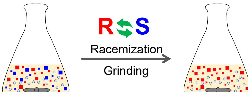
Figure 1.5 Schematic representation of Viedma ripening. The grinding of conglomerate crystals with glass beads coupled with racemization in solution results in solid-phase deracemization.
