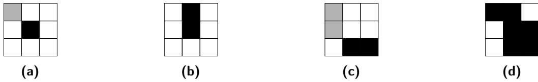
Figure 3.3 – Criterion for pattern identification and extraction: pixels must share at least one border to be considered part of the same pattern. a) Two single events. b) One double event. c) Two double events. d) One multiple event. Different colors indicate different events.
