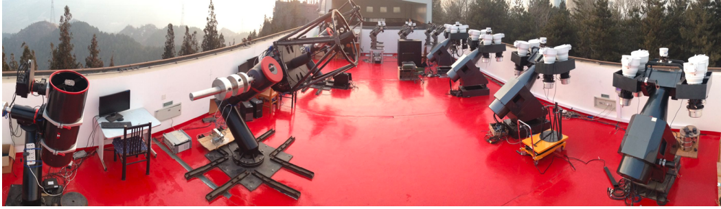
Figure 1.13 – View of the GWAC site. Some of the mounts are visible, as well as the two 60 cm and the single 30 cm telescopes. (NAOC)
