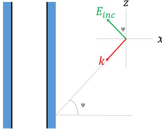
FIGURE 6.23: Cylinder illuminated by an oblique E-polarized plane wave.
