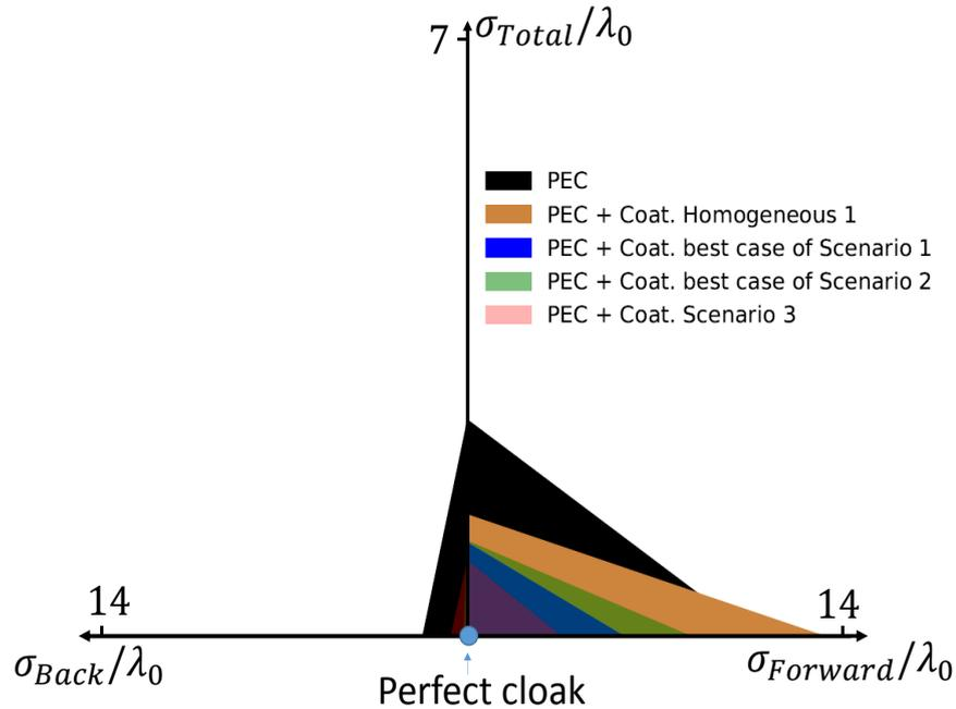
FIGURE 6.15: Triangular representation of  $\sigma_{Back}$ ,  $\sigma_{Forward}$  and  $\sigma_{Total}$  for a PEC cylinder having radius  $a_1 = \lambda/2$ , the PEC coated with the homogeneous coating optimized for back scattering reduction, scenario 3, and the best cases of Scenario 1 and 2.
