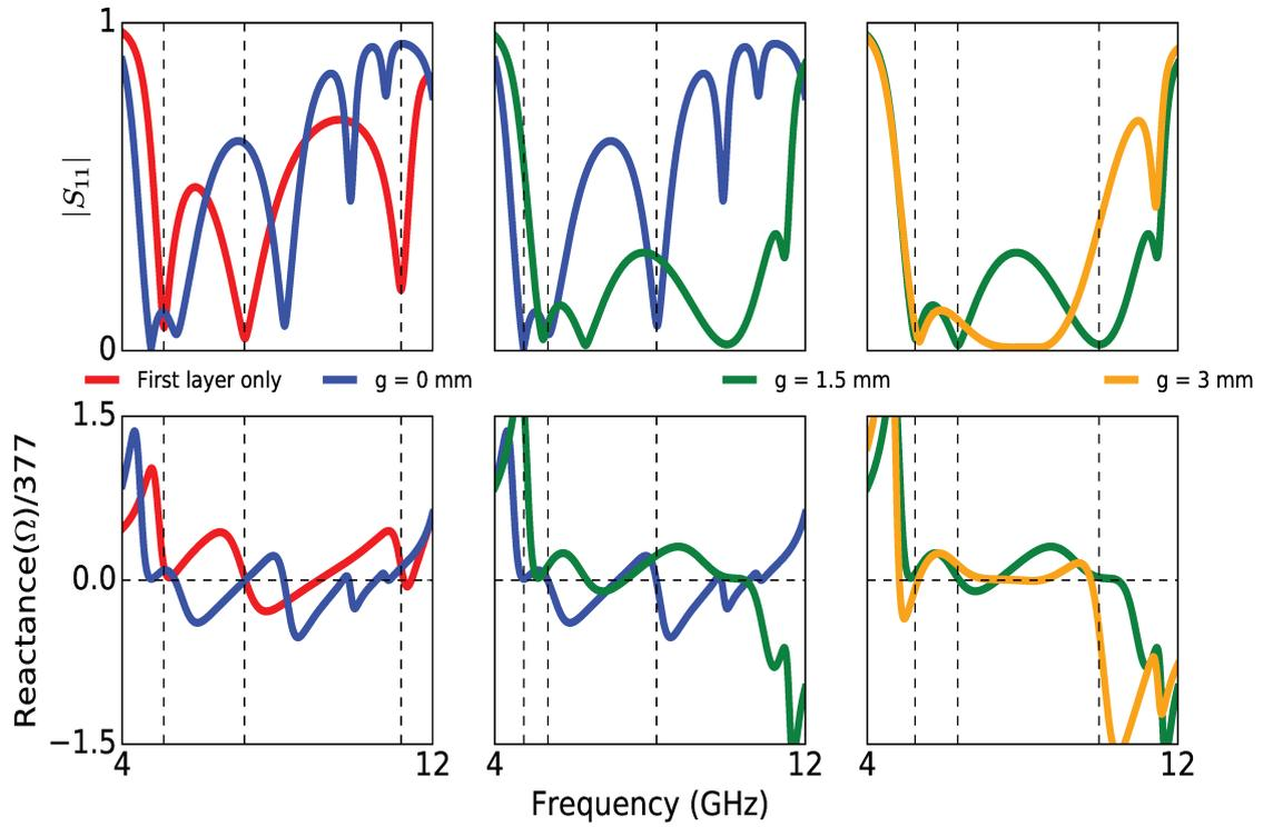
FIGURE 5.4: In the first row, the reflexions ( $S_{11}$ ) of different values of  $g$  are shown. In the second row, the reactances of different values of  $g$  are plotted. Simulations were performed using the commercial software CST Design Studio Suite 2017. Periodic boundary conditions were applied in the numerical model in order to mimic a 2D infinite structure.
