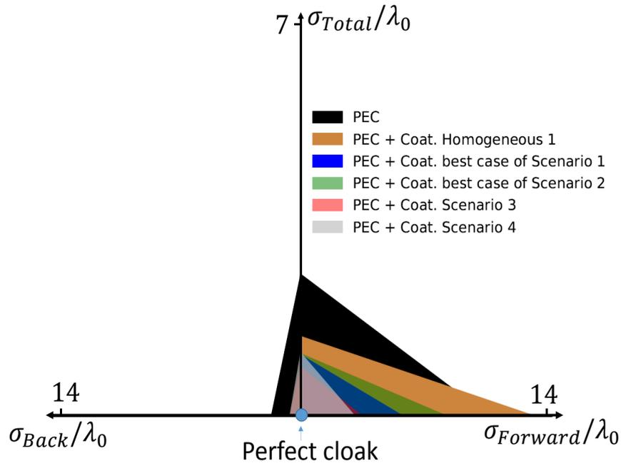
FIGURE 6.18: Triangular representation of  $\sigma_{Back}$ ,  $\sigma_{Forward}$  and  $\sigma_{Total}$  for a PEC cylinder having radius  $a_1 = \lambda/2$ , the PEC coated with the homogeneous coating optimized for back scattering reduction, scenario 4 and the best cases of scenarios 1, 2 and 3.
