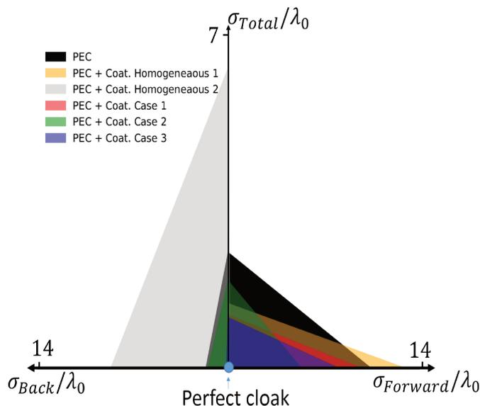
FIGURE 6.10: Triangular representation of  $\sigma_{Back}$ ,  $\sigma_{Forward}$  and  $\sigma_{Total}$  for a PEC cylinder having radius  $a_1 = \lambda/2$ , PEC coated with homogeneous coatings 1 and 2 optimized for back scattering and forward scattering reduction respectively as in Section 6.3.1 and the three cases of inhomogeneous coatings.
