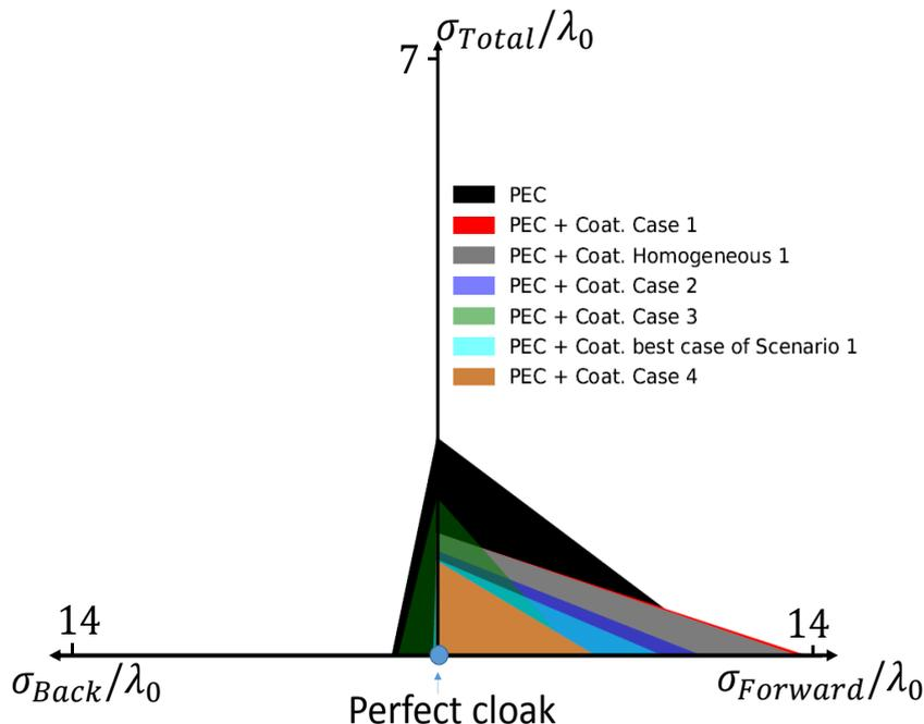
FIGURE 6.13: Triangular representation of  $\sigma_{Back}$ ,  $\sigma_{Forward}$  and  $\sigma_{Total}$  for a PEC cylinder having radius  $a_1 = \lambda/2$ , the PEC coated with the homogeneous coating optimized for back scattering reduction, four cases of scenario 2 and the best case of scenario 1.
