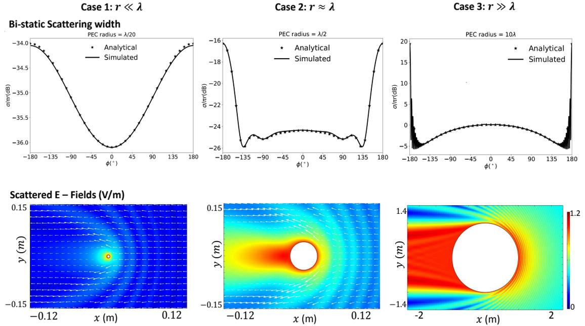
FIGURE 6.2: First row: Analytical and Simulated normalized (with respect to  $\pi r$ ) scattering widths of PEC cylinders for the three cases. Second row: Scattered electric field from the PEC cylinders. An illumination of E polarized wave is considered. Simulations and calculations were done for 3 GHz.
