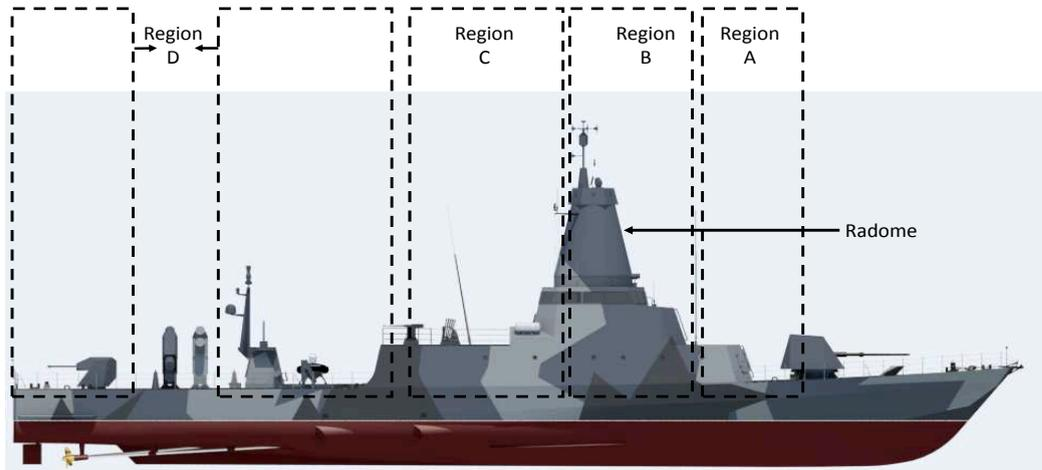
FIGURE 1.1: Profile view of the Combattante FS56. Regions A, B, C and D are regions where antennas and radars are placed.
