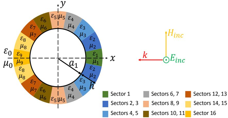
FIGURE 6.19: PEC cylinder having radius  $a_1 = \lambda/2$  coated by 16 sectors dielectrics having a thickness  $h = \lambda/5$  illuminated by an E-polarized plane wave.
