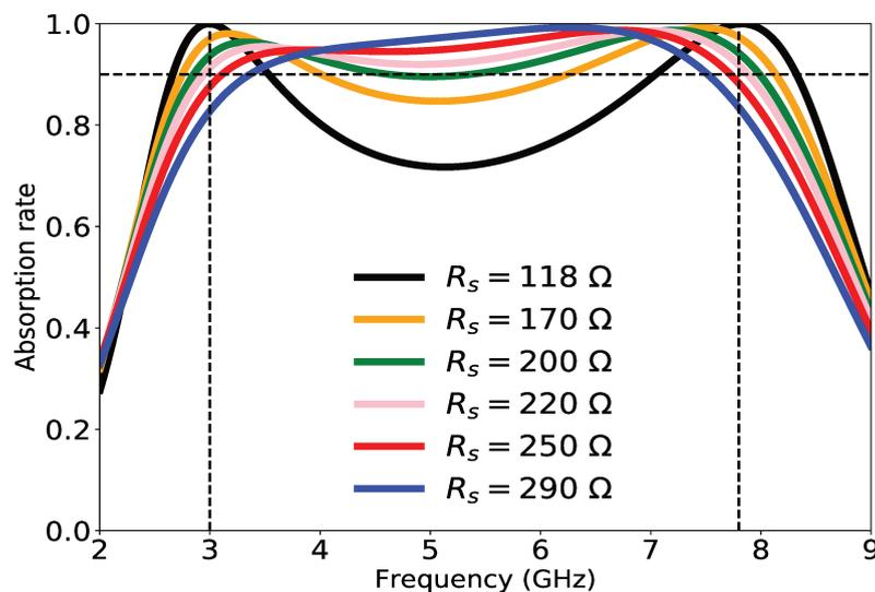
FIGURE 3.4: Absorption rate for different values of resistance.
