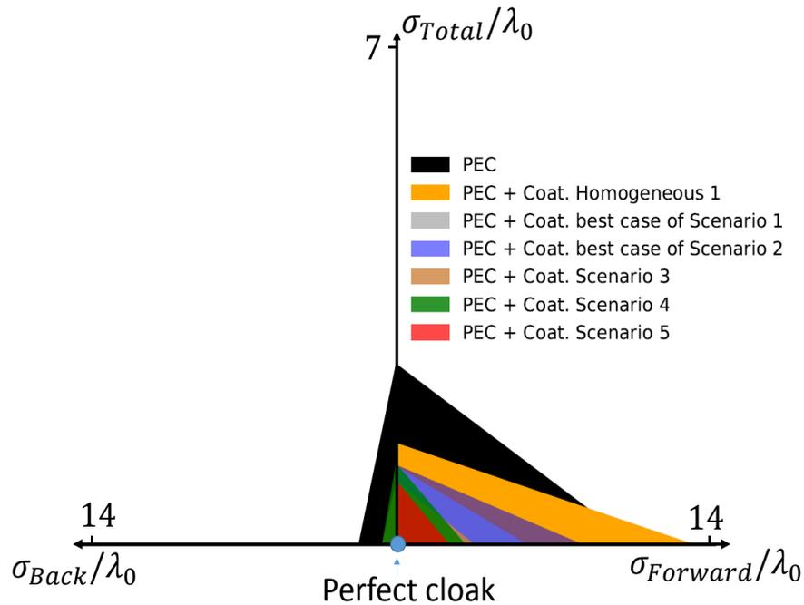
FIGURE 6.21: Triangular representation of  $\sigma_{Back}$ ,  $\sigma_{Forward}$  and  $\sigma_{Total}$  for a PEC cylinder having radius  $a_1 = \lambda/2$ , scenario 4 and the best cases of scenarios 1, 2 and 3.
