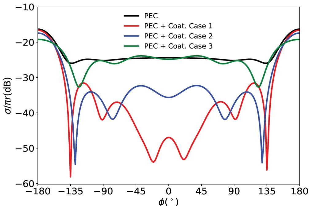
FIGURE 6.9: Bi-Static scattering for a PEC cylinder having radius  $\lambda/2$  (black), the case when Sector 1 is lossy (red), the case when Sector 1 is not lossy (green) and the intermediate case (blue). Sector 2 is fixed in the three for the three cases. An illumination of E polarized wave is considered. Simulations and calculations were done for 3 GHz.
