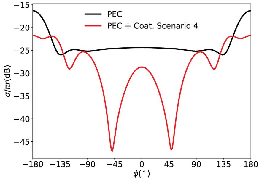
FIGURE 6.17: Bi-Static scattering for a PEC cylinder having radius  $\lambda/2$  (black) and for Scenario 4 (red). An illumination of E polarized wave is considered. Simulations and calculations were done for 3 GHz.
