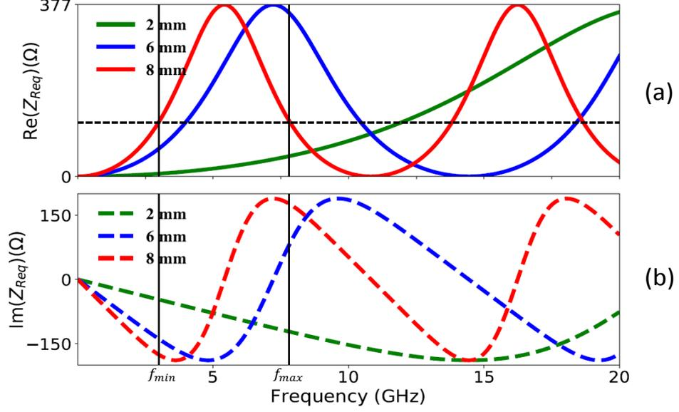
FIGURE 3.1: (a): Real part of required impedance of the complex sheet. (b): Imaginary part of required impedance of the complex sheet. The two solid vertical black lines represent the  $f_{min} = 3$  GHz and  $f_{max} = 7.8$  GHz limits which is our frequency band design goal. The required impedance have been plotted using Equations 2.8 - 2.10 of Chapter 2. Note that  $Z_{Req}$  was called  $Z_{sr}$  in Chapter 2.
