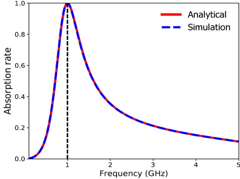
FIGURE 2.13: Analytical and numerical (simulated) absorption rates.
