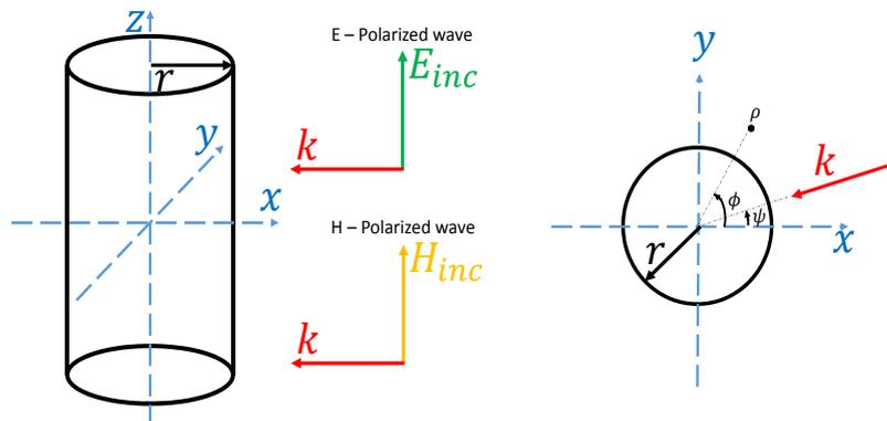
FIGURE 6.1: Illustration of a perfectly conducting cylinder illuminated by electromagnetic plane waves and the associated polar system with incidence and scattering angles.
