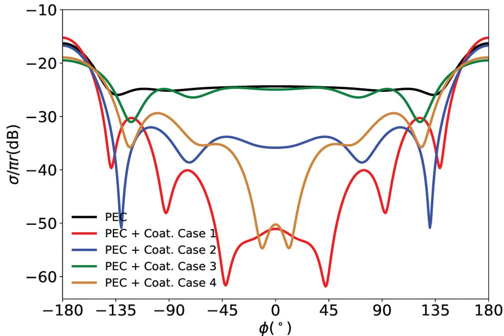
FIGURE 6.12: Bi-Static scattering for a PEC cylinder having radius  $\lambda/2$  (black) and for the for different cases. An illumination of E polarized wave is considered. Simulations and calculations were done for 3 GHz.
