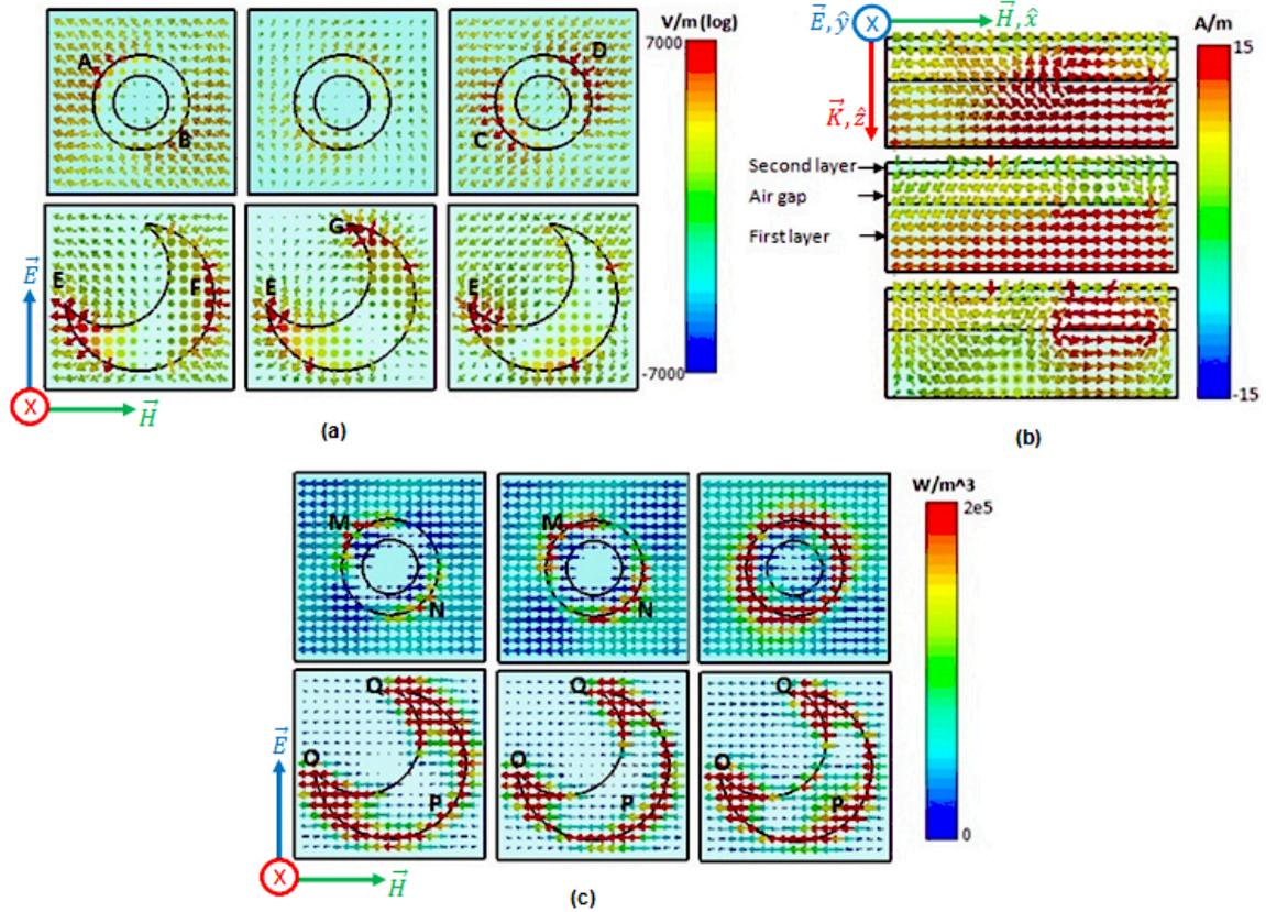
FIGURE 5.10: (a) Top view of electric field distribution on the first and second layers. (b) Perspective view of magnetic field distribution on the first whole structure. (c) Top view of power loss density on the first and second layers.
