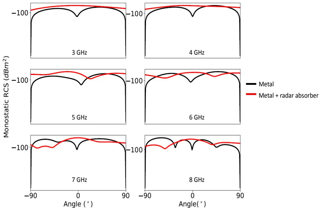
FIGURE 3.14: Cross-polarization Monostatic RCS at 3, 4, 5, 6, 7 and 8 GHz of the absorbing structure and a perfectly conducting plate of the same dimensions.
