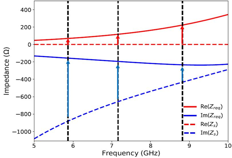
FIGURE 4.8: Required real ( $\text{Re}(Z_{req})$ ) and imaginary ( $\text{Im}(Z_{req})$ ) parts of surface impedance for perfect absorption of a 3.2 mm FR4 grounded dielectric and actual real ( $\text{Re}(Z_s)$ ) and imaginary ( $\text{Im}(Z_s)$ ) parts of the impedance of the UUSR.
