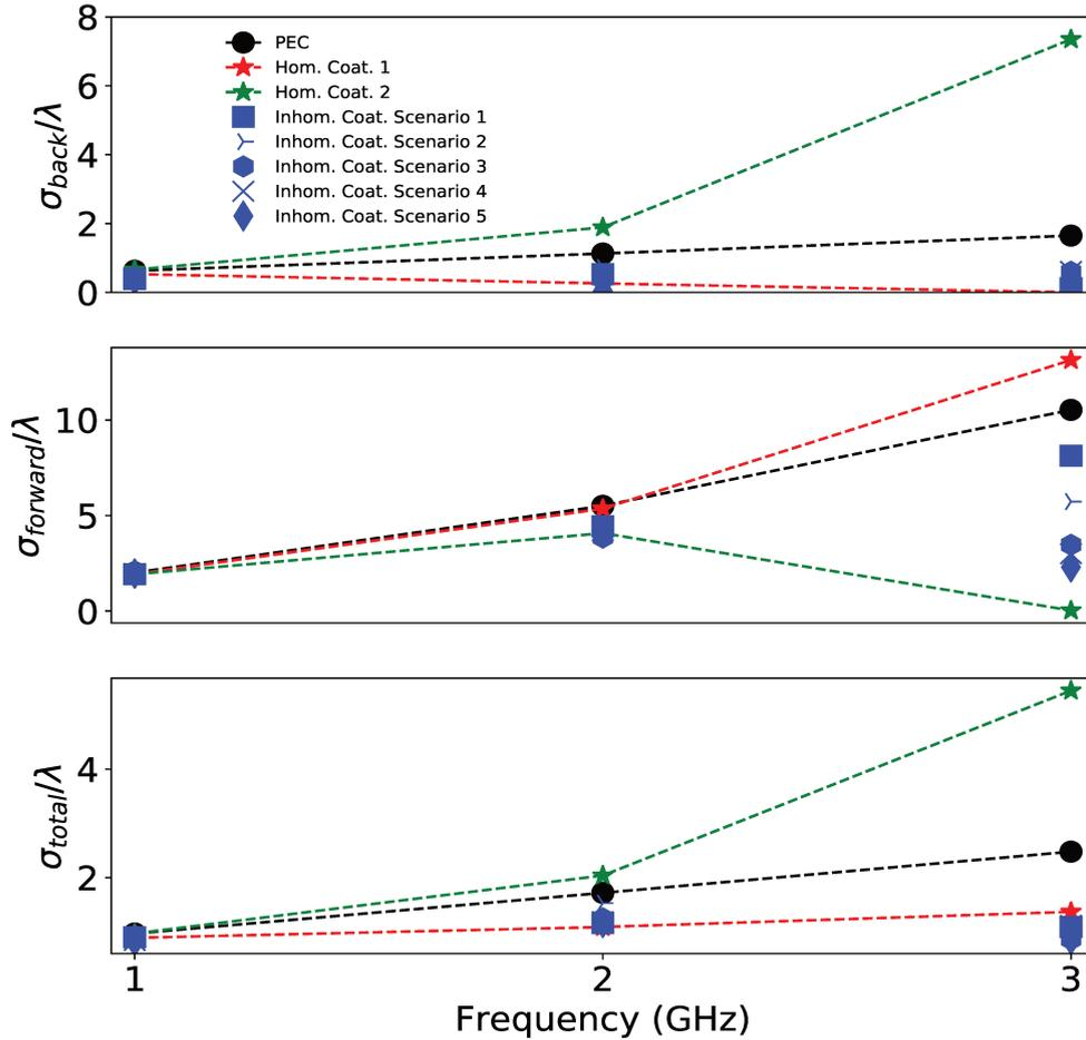
FIGURE 6.22: Frequency dependency of scattering of a PEC cylinder having radius  $a_1 = \lambda/2$  and the PEC cylinder coated with homogeneous and inhomogeneous coatings. On top: The normalized back scattering width is presented. In the middle: The normalized forward scattering width is shown and on the normalized total scattering width is shown on the bottom. An illumination of E polarized wave is considered in all the cases. Simulations have been done at 1, 2 and 3 GHz.
