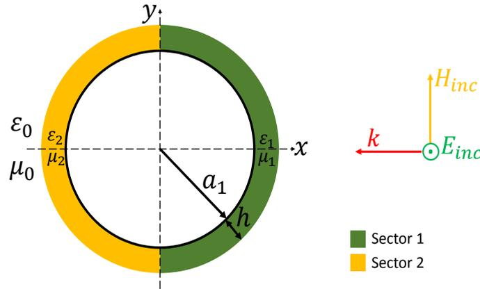
FIGURE 6.8: PEC cylinder having radius  $a_1 = \lambda/2$  coated by two sectors having a thickness  $h = \lambda/5$  illuminated by an E-polarized plane wave.
