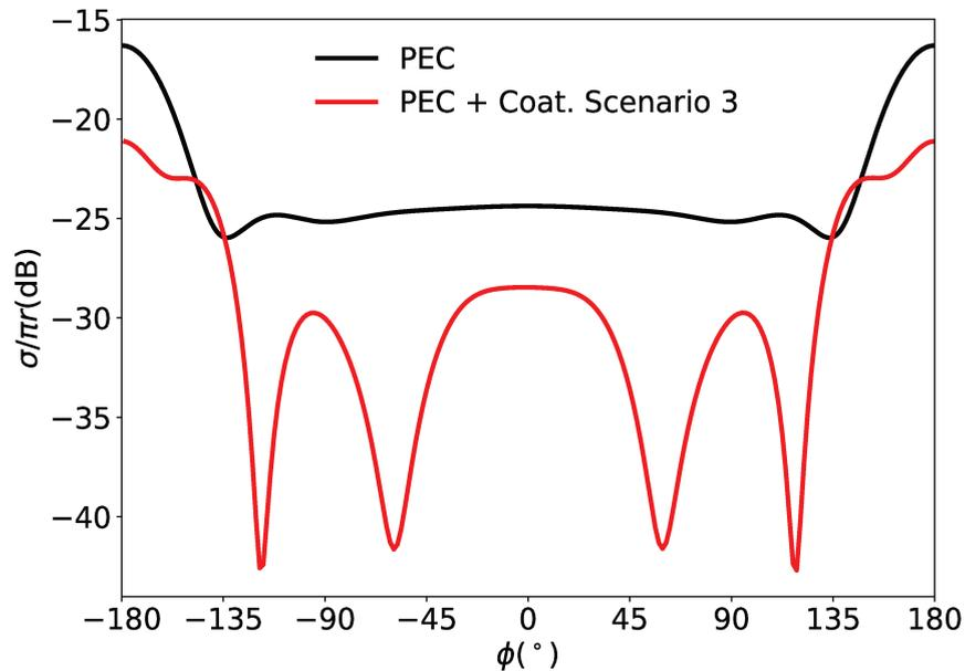
FIGURE 6.14: Bi-Static scattering for a PEC cylinder having radius  $\lambda/2$  (black) and for Scenario 3 (red). An illumination of E polarized wave is considered. Simulations and calculations were done for 3 GHz.
