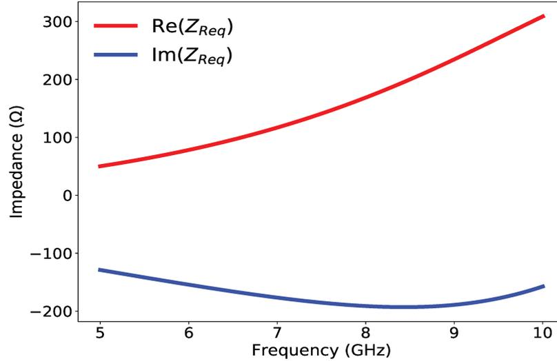
FIGURE 4.1: Required real ( $\text{Re}(Z_{req})$ ) and imaginary ( $\text{Im}(Z_{req})$ ) parts of surface impedance for perfect absorption of a 3.2 mm FR4 grounded dielectric substrate having a permittivity of 3.92 and loss tangent of 0.025. A normally incident linearly polarized TE wave is considered.
