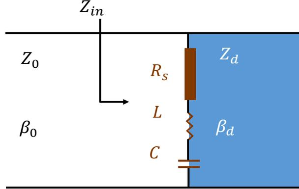
FIGURE 3.2: TLM model proposed for broadband absorption.
