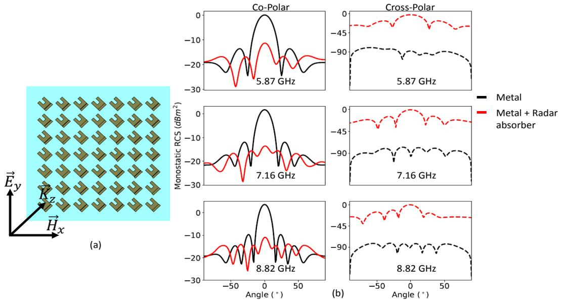
FIGURE 4.12: (a) Simulated normally arranged full structure. (b) Monostatic RCS for 5.87, 7.16 and 8.82 GHz of the absorbing structure and a perfectly conducting plate of the same dimensions. The first column represents co-polarization RCS results and the second column represents results for cross-polarization RCS.
