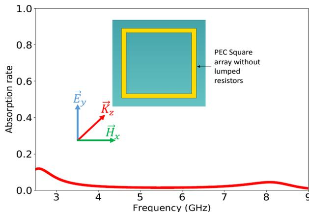
FIGURE 3.6: Simulated absorption rate of the radar absorber. The PEC square arrays are continuous (without lumped resistors). A normal incident linearly polarized TE wave is considered. Same results are obtained for TM mode.
