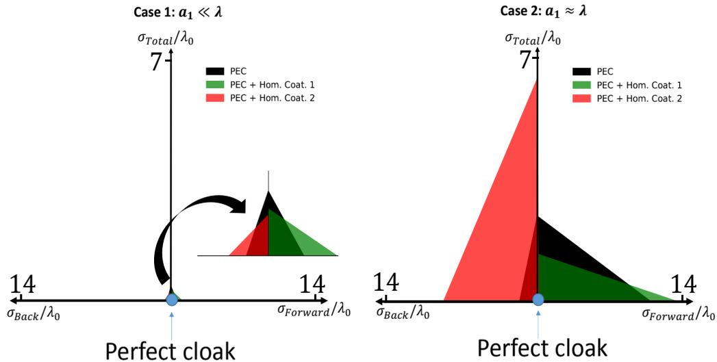
FIGURE 6.7: Triangular representation of  $\sigma_{Back}$ ,  $\sigma_{Forward}$  and  $\sigma_{Total}$ . The radius of the PEC cylinder (black triangles) is  $a_1 = \lambda/20$  for Case 1, and  $a_1 = \lambda/2$  for Case 2.
