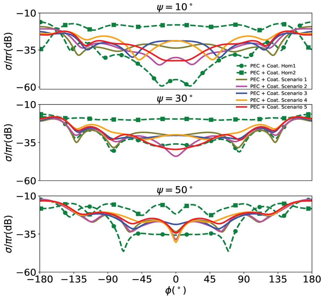
FIGURE 6.24: Normalized scattering widths under oblique incidences of a PEC cylinder having radius  $a_1 = \lambda/2$  coated with homogeneous and inhomogeneous coatings of thickness  $\lambda/5$ . Simulations have been done at 3 GHz.
