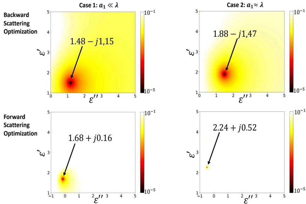
FIGURE 6.4: Colormap to find real and imaginary parts of the permittivity to have the minimum possible backward scattering and forward scattering at 3 GHz for the cases when  $a_1 \ll \lambda$  and  $a_1 \approx \lambda$ . For  $a_1 \ll \lambda$  and  $a_1 \approx \lambda$ , the radius of the PEC cylinder is of  $\lambda/20$  and  $\lambda/2$  respectively.
