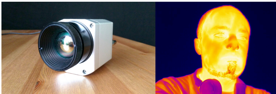
FIGURE 3.4: The Optris PI640 thermal camera and an example of a thermal image representation
