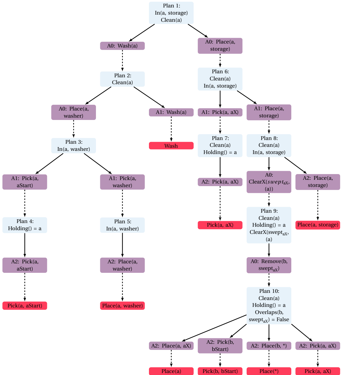
Fig. 4.2 Planning and execution tree for washing and storing an object. The wildcard character * replaces any free space where an object could be placed
