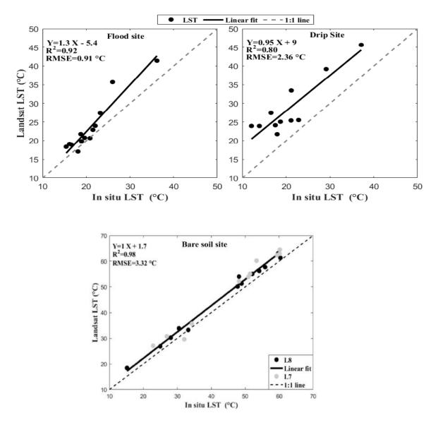
Figure II.8: LST derived from Landsat-7 and -8 versus in situ measurements for R3 two drip (top right) and flood (top left) irrgated sites and Sidi Rahal bare soil site (bottom).
