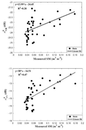
Fig. 5. Radar signal sensitivity to SM for VH (top) and VV (bottom) polarization over the Sidi Rahal site.
