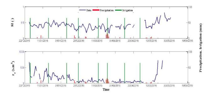
Figure IV.2: Variations of SI (top figure) and r<sub>c</sub> (bottom figure) under different water stress conditions for the R3- flood wheat site. Rainfall (green vertical lines) and irrigation (red vertical lines) events are scaled on the secondary y-axis.
