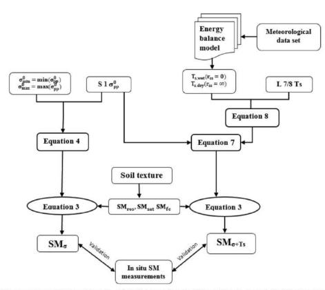
Fig. 3. Flowchart for the benchmark (radar only, on the left) and new (combined thermal and radar, on the right) SM retrieval approaches.
