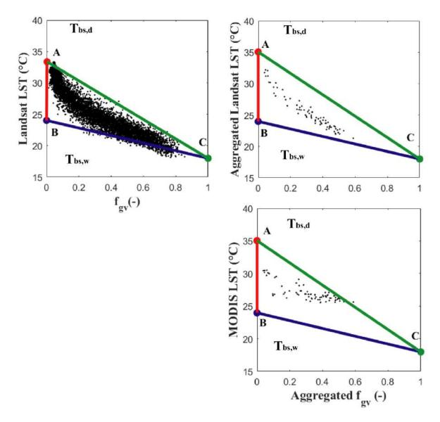
Figure III.1: Scatterplot of LST- $f_{gv}$  spaces at 100 m (left) and 1 km (right) resolution on February 07. In the LR case, extreme temperatures are estimated using a soil energy balance (EB) model over R3 site.
