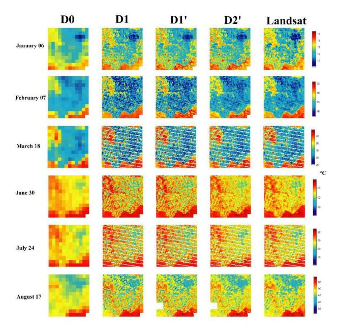
Figure IV.11: Maps of the LR (Landsat-aggregated) LST disaggregated by the four algorithms compared to the Landsat reference HR LST on six selected clear dates separately over Sidi Rahal area.
