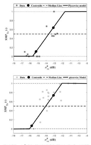
Fig. 6.  $SMP_{Ts} - \sigma_{vv}^0$  relationship using  $T_s$  derived from Landsat data over Sidi Rahal (top plot) and R3 (bottom plot) site. The solid line represents the assumed piecewise linear model.
