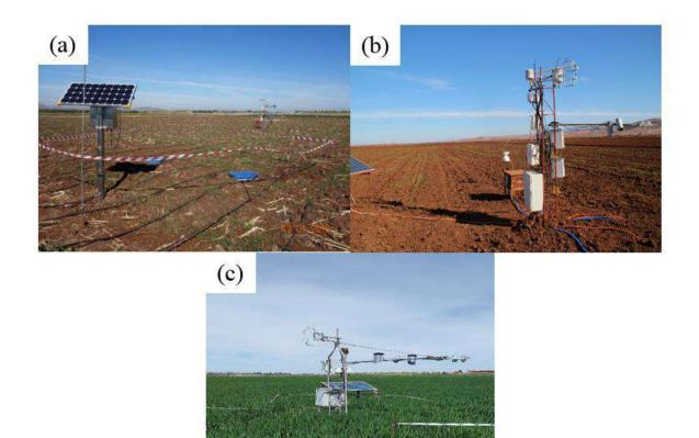
Figure II.6: Flux stations over (c) flood, (a) drip irrigated sites and (b) Sidi Rahal bare soil during the 2016 growing season.
