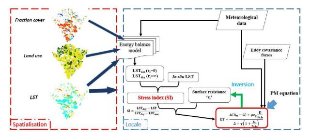
Figure III.2: Flowchart of the retrieval approach to estimates LE using locale and spatial data acquired from Landsat.
