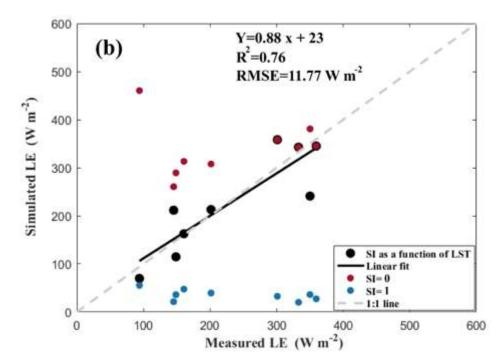
Figure IV.10: Comparison between the simulated and measured LE ( $W m^{-2}$ ) over flood (a) and drip (b) sites in different conditions (un-stressed condition "SI = 0"; "stressed condition "SI = 1"; real condition "SI as a function of LST").
