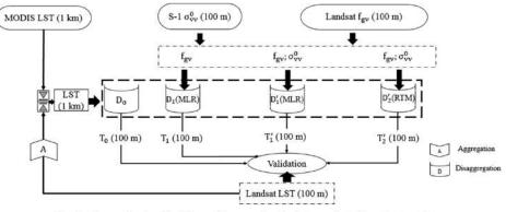
Fig. 3. Diagram showing the different disaggregation algorithms and their input/output data.
