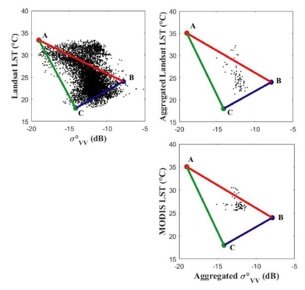
Figure III.6: Scatterplot of  $LST-\sigma_{vv}^0$  spaces at 100 m (left), aggregated Landsat temperature to 1 km (right) and MODIS-LST at 1 km (bottom) resolution on February 07. In the low resolution case, extreme temperatures are estimated using a soil EB model over R3 site.
