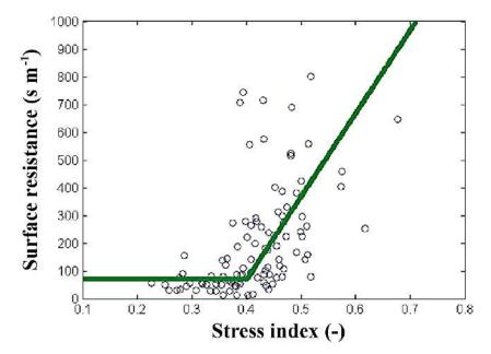
*Figure IV.3: Relationship between the bulk surface resistance* (*r<sub>c</sub>*) *and a stress index* (*SI*) *for the flood irrigated parcel. The best fit (green solid line) was presented.*
