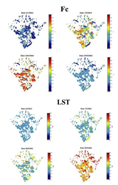
Fig. 7 — Time series of fraction cover (Fc) and Land Surface Temperature (LST) maps over R3 area at dates corresponding to different growing stages obtained from Landsat satellite.
