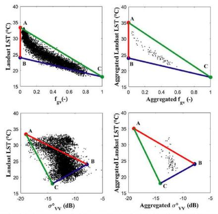
Fig. 5. Scatterplot of LST-fgv and LST- $\sigma_w^0$  spaces at 100 m (left) and 1 km (right) resolution. In the LR case, extreme temperatures are estimated using a soil EB model on February 07 over R3 site.
