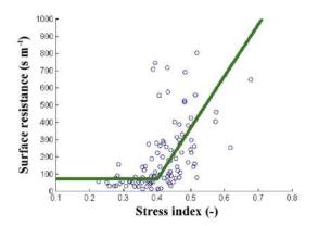
Fig. 5 – Relationship between the bulk surface resistance  $(r_c)$  and a stress index (SI) for the flood irrigated parcel. The best fit (green solid line) was presented. (For interpretation of the references to colour in this figure legend, the reader is referred to the web version of this article.)
