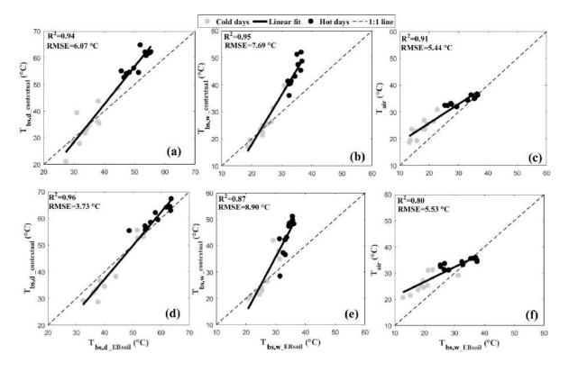
*Figure IV.1: EB-simulated versus space-based soil temperature endmembers (T<sub>bs,w</sub> and T<sub>bs,d</sub>) for R3 (a, b, c) and Sidi Rahal (d, e, f) sites separately.*
