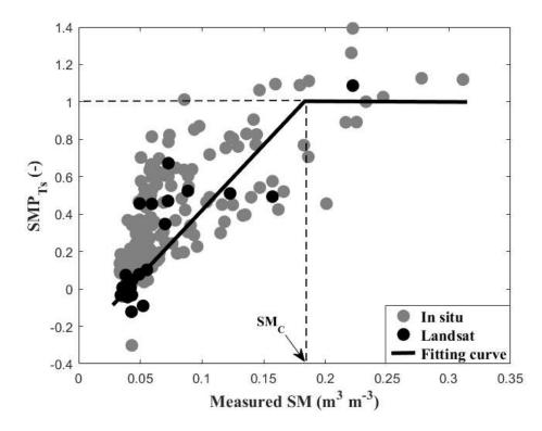
Figure III.4: The SMP<sub>Ts</sub> (Eq III.1) derived from 1) in situ LST data collected at 11:00 am (Landsat overpass time) and 2) L7/8 LST-derived data is plotted as a function of in situ SM (Measured SM) at Sidi Rahal site.
