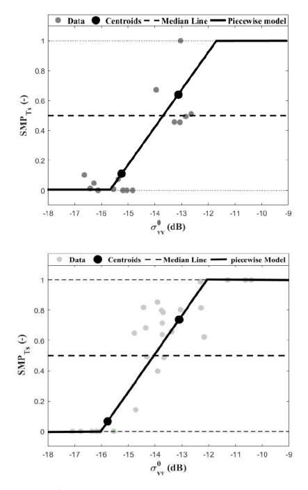
Figure IV.18:  $SMP_{Ts} - \sigma_{vv}^0$  relationship using  $T_s$  derived from Landsat data over Sidi Rahal (top plot) and R3 (bottom plot) site. The solid line represents the assumed piecewise linear model.
