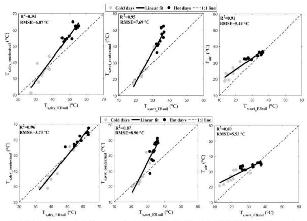
Fig. 9. EB-simulated versus space-based soil temperature endmembers (T<sub>s,wet</sub> and T<sub>s,dry</sub>) for R3 (top plots) and Sidi Rahal (bottom plots) sites separately.
