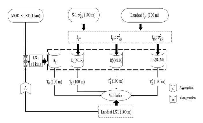
Figure III.7: Diagram showing the tow disaggregation algorithms and their input/output data.
