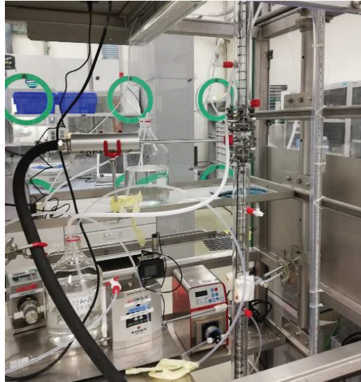
Figure 6.1: Lab-scale pulsed column with the SOPAT probe
