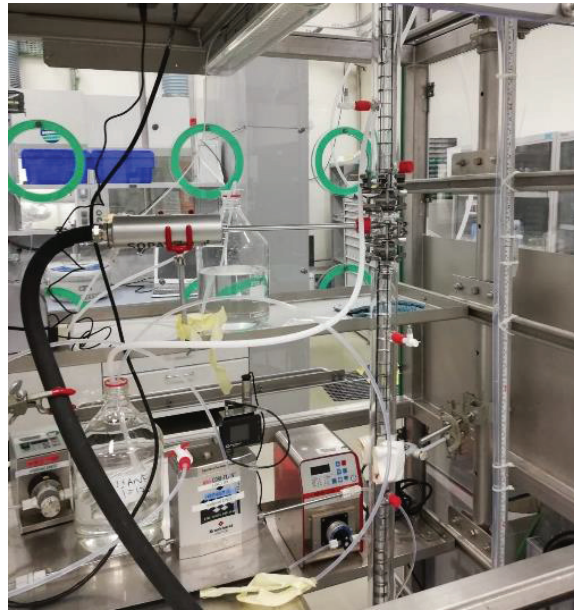
Figure 3.6: Lab-scale pulsed column
