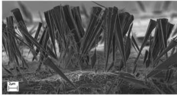
Figure 1.13: SEM image of the diamond needles after selective oxidation of the (001) textured polycrystalline CVD film.
