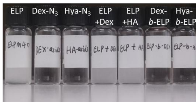
Turbidity comparison at 125 \mu M 35°C ( Physical mixture vs Covalent conjugate)
