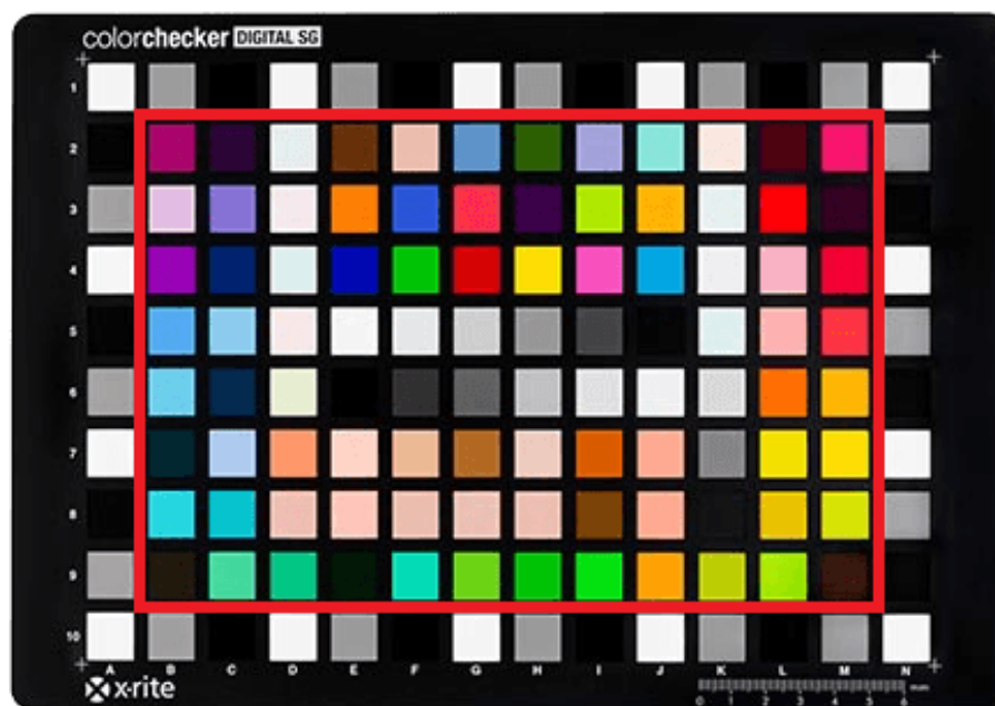
FIGURE 5.5 – X-Rite ColorChecker® Digital SG (issue de https://www.xrite.com/categories/calibration-profiling/colorchecker-digital-sg ).
