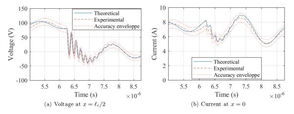
Figure 4.18 – Validation results for the RL series C parallel load, zoom on the 6, 4MHz resonance
