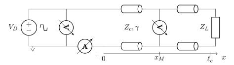
Figure 4.8 – Schematic for the time domain validation experiment
