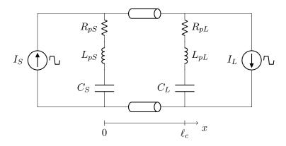
Figure 5.17 – Schematic of the simulated model of the DC link with voltage elevation
