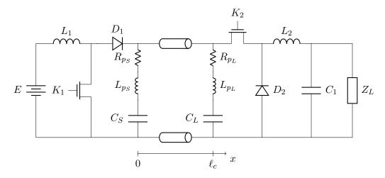
Figure 5.15 – Schematic of the DC link with voltage elevation: boost converter at the cable input and buck converter at the cable output
