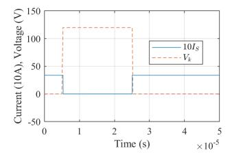
Figure 5.29 – Sources  $I_S$  and  $V_k$  — approximated as ideal trapezoidal sources
