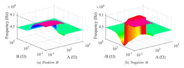
Figure C.5 – Resonance frequency in function of  $Z_L = A + jB$ , cable of section  $1.5 mm^2$
