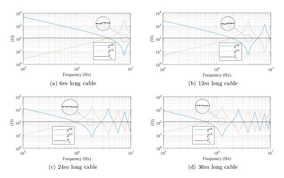
Figure 2.10 – Two-conductor cable characteristic impedance identification for different lengths
