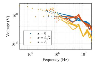
Figure 4.16 – The voltage along the line on the frequency domain
