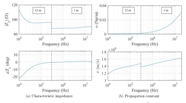
Figure 2.30 – Parameters of the cable of section  $0.75 \, mm^2$
