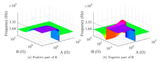
Figure C.11 – First resonance frequencies of the two-conductor  $2.5\,mm^2$  cable of length  $200\,m,$  in function of the load
