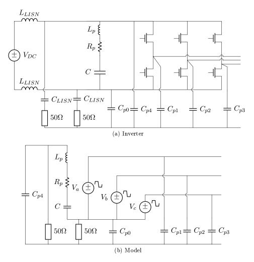
Figure 5.6 – Two-level inverter model, with LISN
