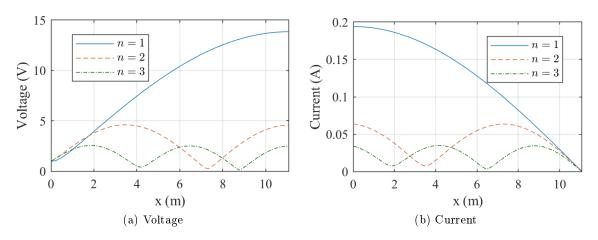
Figure 2.36 – Voltage and current envelopes of an open-ended resonant line
