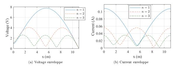
Figure 2.35 – Voltage and current envelopes of a short-circuited resonant line
