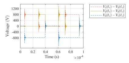
Figure 5.14 – Phase-to-phase voltages at  $x = \ell_c$  for  $\ell_c = 12 m$
