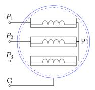
Figure I.1 – Schematic of the three-phase motor as a 4 input device
