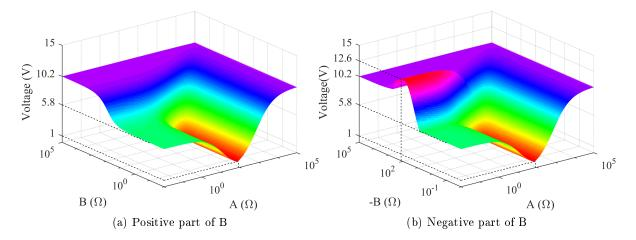
Figure C.8 – Maximal voltage amplification of the two-conductor  $2.5 mm^2$  cable of length 50 m, in function of the load
