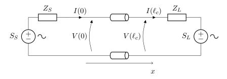
Figure 2.3 – Schematic of the generalized frequency domain model for two-conductor cables
