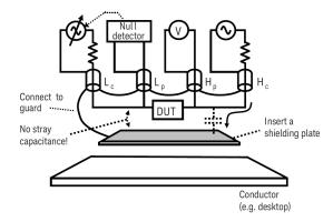
Figure 2.12 – Solution to avoid common-mode-due error [21]
