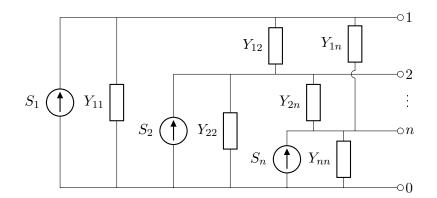
Figure 3.3 - (n+1)-port equivalent circuit
