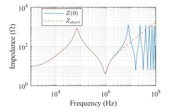
connected to an LC load is predicted simply by circuit theory, the long transmission line model, with distributed parameters, is necessary to predict the complete resonance behavior of a cable.
