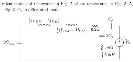
Figure 5.35 – System equivalent circuit in common mode
