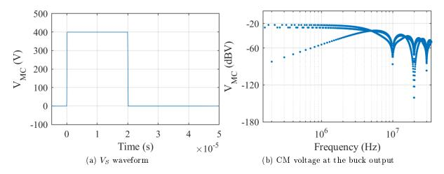
Figure 5.37 – Simulation of the CM voltage generated by the buck converter
