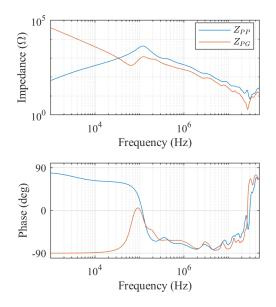
Figure H.5 – Impedances  $Z_{PP}$  and  $Z_{PG}$ , measured with impedance analyzer
