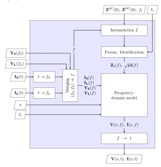
Figure 4.5 – Flowchart of the complete model
