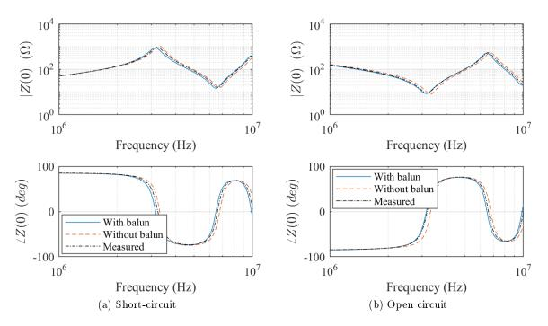
Figure 2.25 – Input impedance comparison, theoretical calculations using parameters obtained from identification with and without balun
