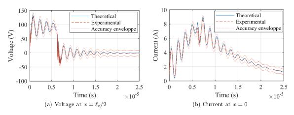
Figure 4.17 – Vatidation results for the RL series C parallel load
