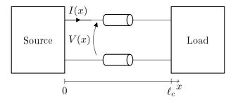
Figure 2.1 – Two-conductor transmission line, variable definition
