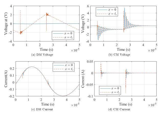
Figure 5.31 – Voltages and currents at the line extremities with  $C_2 = C_3 = 22 \, pF$ , without DC component
