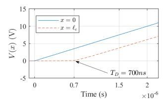
Figure 4.27 – Voltage pulse sent into a  $\ell_c = 100 m$  long cable
