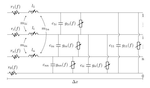
Figure 4.3 – Basic cell for time domain simulation of a MTL, parameter variable on frequency
