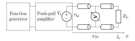
Figure 2.19 – Schematic of the validation resonance-based experiment
