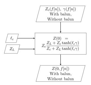
Figure 2.24 – Theoretical input impedande caculation
