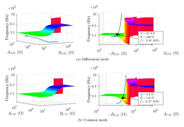
Figure 3.27 – Intersection of the modal impedances with the resonance frequency surfaces.
