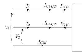
Figure 3.21 – Differential and common-mode currents
