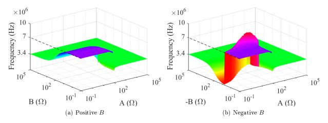
Figure C.2 – Resonance frequency in function of  $Z_L = A + jB$ , cable of section  $0.75 \, mm^2$
