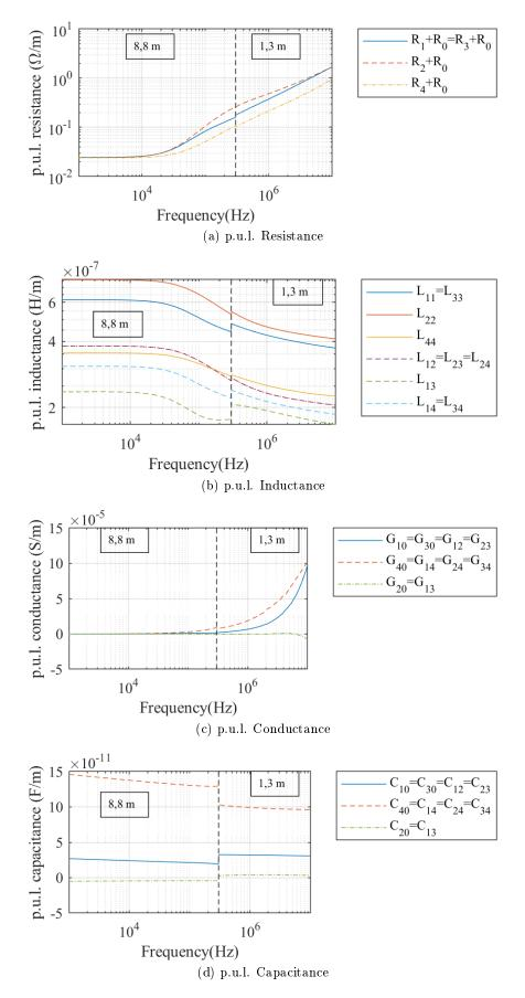
Figure G.2 – Parameters of the shielded cable with 4 conductors of section  $1.5 \, mm^2$
