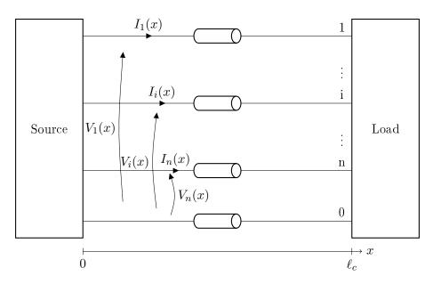
Figure 4.4 – Schematic of the multiconductor transmission line
