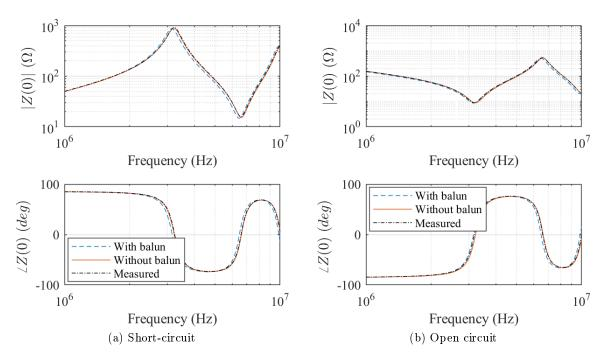
Figure 2.26 – Input impedance comparison, theoretical calculations using parameters obtained from identification with or without balun, identification without balun on ideal configuration
