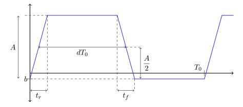
Figure 4.6 – Parameters of periodical trapezoidal source
