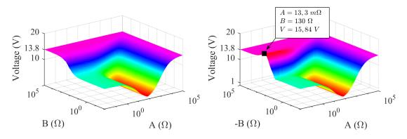
Figure 2.45 – The maximum voltage amplification possible due to resonance phenomena
