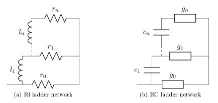
Figure 4.1 – T-ladder network to represent the cable losses
