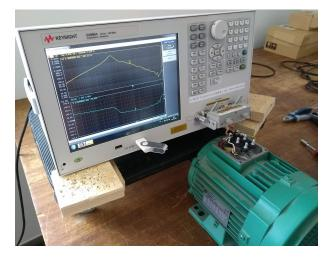
Figure H.2 – Motor input impedance measurement setup
