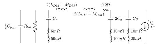
Figure 5.36 – Switching device equivalent circuit in differential mode
