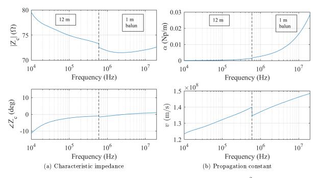
Figure 2.32 – Parameters of the cable of section  $2.5\,mm^2$
