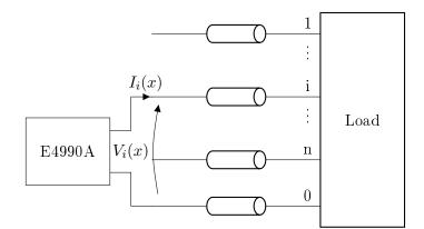
Figure 3.7 – Self impedance measurement setup
