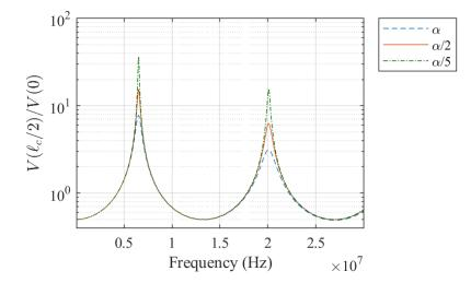
Figure 2.37 – Voltage envelope in function of frequency for the short-circuited two-conductor cable of section 2.5 mm2, with variations on the attenuation constant  $\alpha$
