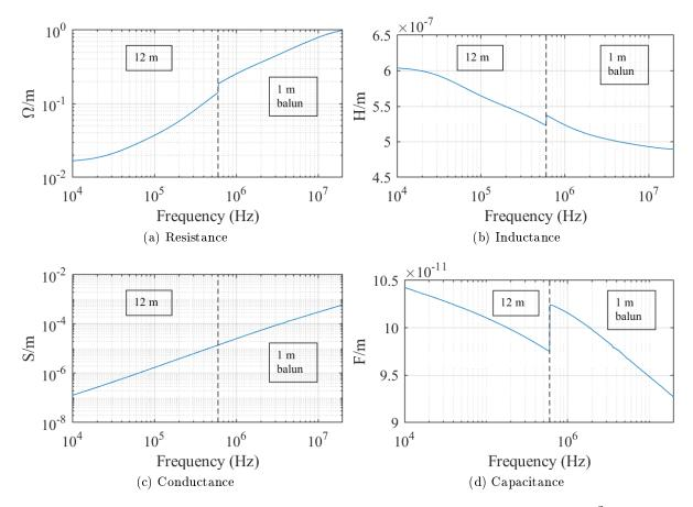
Figure 2.33 – Per-unit-length parameters of the cable of section  $2.5 \, mm^2$
