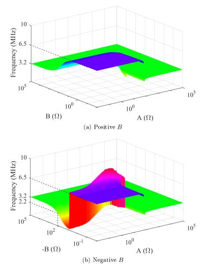
Figure 2.40 – Resonance frequency in function of  $Z_L = A + jB$ , positive and negative parts of B
