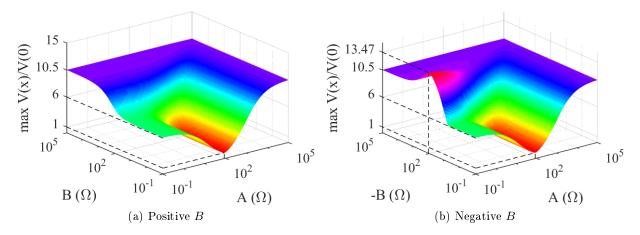
Figure C.1 – Maximum voltage in function of  $Z_L = A + jB$ , cable of section  $0.75 mm^2$
