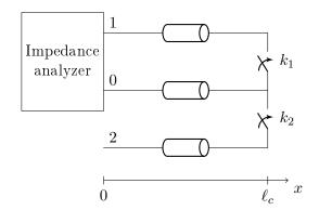
Figure 3.14 – Schematic: input impedance validation experiment
