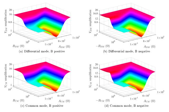
Figure 3.23 – Voltage amplification due to resonance on the three-conductor cable, in differential and common mode, in function of the modal load
