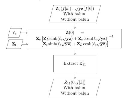
Figure 3.15 – Theoretical input impedance calculation
