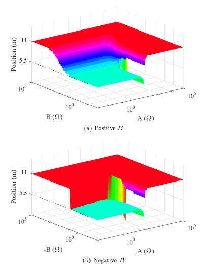
Figure 2.41 – Position of the maximum voltage in function of  $Z_L = A + jB$ , positive and negative parts of B
