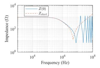
Figure 2.51 – Input impedance of the open-ended line
