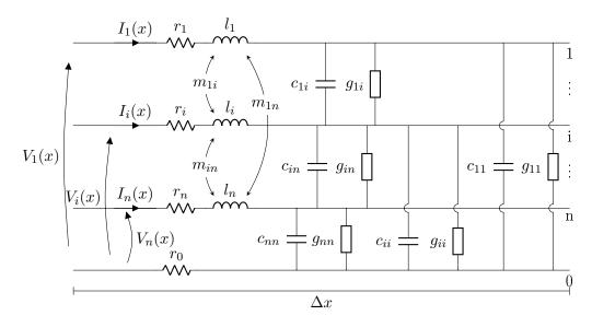
Figure 3.2 – Elementary cell of multiconductor transmission lines, with its p.u.l. parameters
