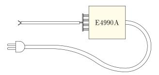
Figure 2.15 – Configuration "B": common-mode enhancing configuration
