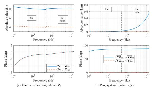
Figure 3.18 – Three-conductor cable complex parameters
