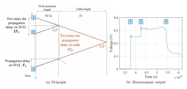
Figure 2.7 – Time-domain reflectometer (TDR)
