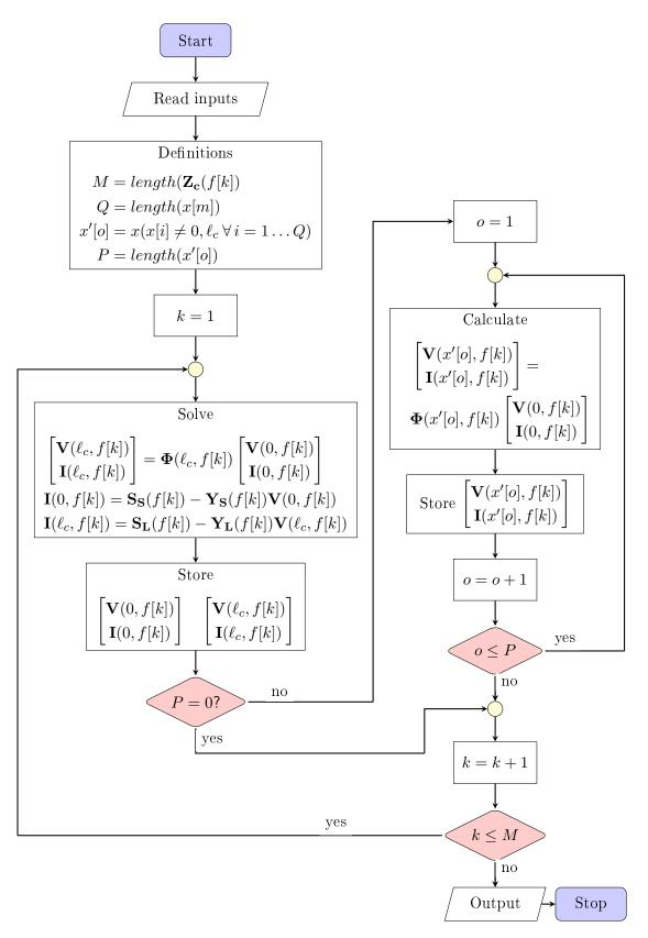
Figure 3.6 – Program flowchart of the frequency domain simulation tool — multiconductor cables
