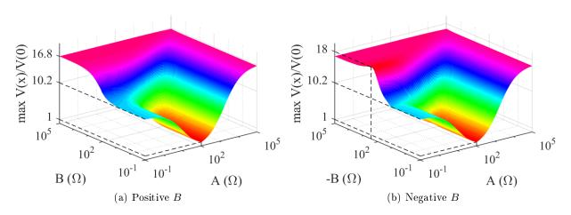
Figure C.4 – Maximum voltage in function of  $Z_L = A + jB$ , cable of section  $1.5 mm^2$
