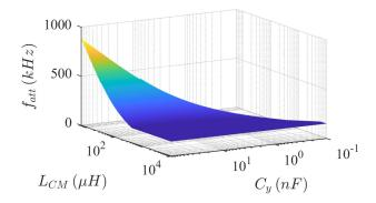
Figure 5.39 – Frequencies of the maximum in common mode
