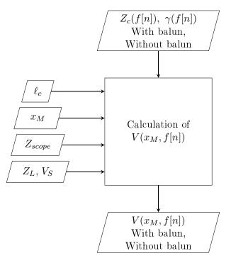
Figure 2.22 – Frequency domain voltage simulation
