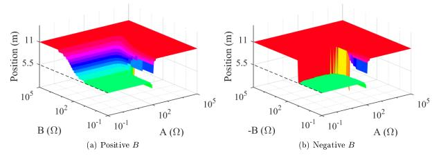
Figure C.6 – Position of the maximum voltage in function of  $Z_L = A + jB$ , cable of section  $1.5 mm^2$
