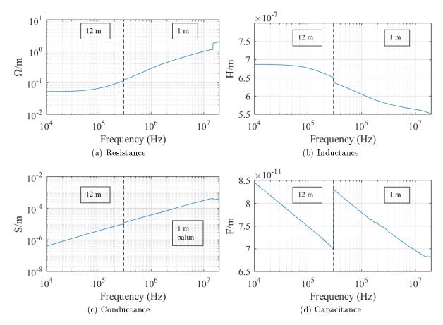
Figure 2.31 – Per-unit-length parameters of the cable of section  $0.75 \, mm^2$
