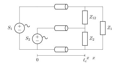
Figure 3.22 – Schematic for numerical resonance analysis,  $\ell_c = 12 m$
