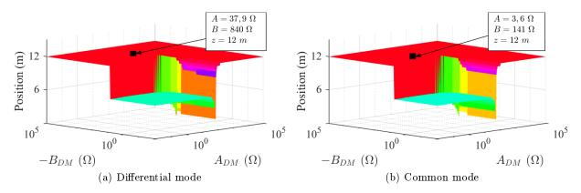
Figure 3.29 - Points of intersection on the position of maximal amplification due to resonance surfaces
