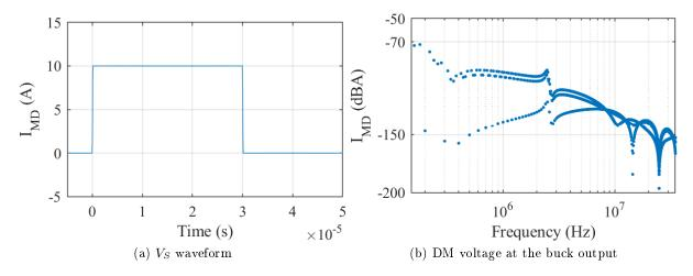
Figure 5.41 - Simulation of the DM current generated by the buck converter with common mode
