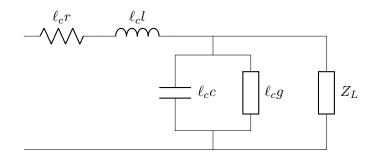
Figure 2.48 – Representation of an electrically short line, with load  $Z_L$
