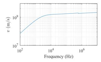
Figure 4.28 – Propagation speed in the  $2.5 mm^2$  two-conductor cable
