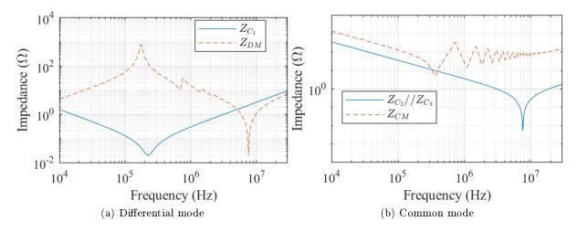
Figure 5.27 – Comparison between the input impedances of the system and the capacitive part of the filter
