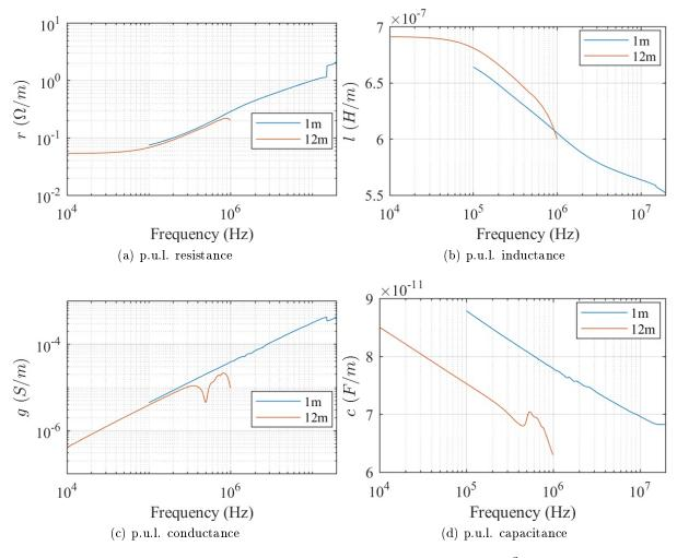
Figure 2.28 – Per-unit-length parameters of the  $0.75 \, mm^2$  cable
