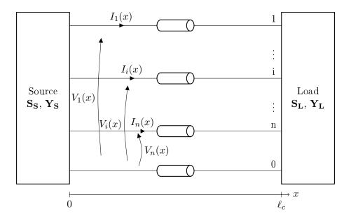
Figure 3.4 – Multiconductor transmission line, variables definition
