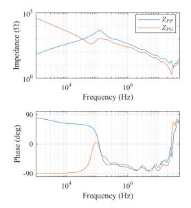
Figure 5.3 – Motor Leroy Somer  $1.5 \, kW$  measured impedances
