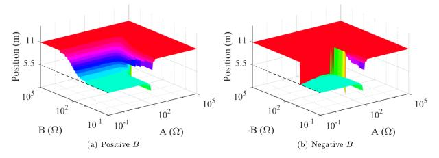
Figure C.3 – Position of the maximum voltage in function of  $Z_L = A + jB$ , cable of section  $0.75 mm^2$
