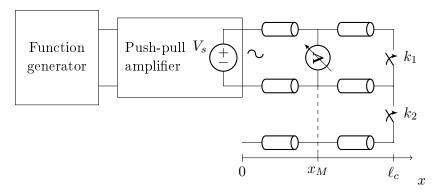
Figure 3.10 – Schematic: resonance-based validation experiment
