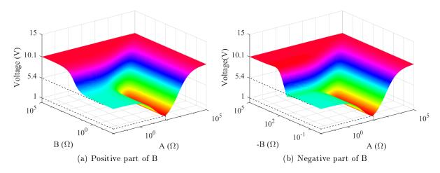
Figure C.10 – Maximal voltage amplification of the two-conductor  $2.5\,mm^2$  cable of length  $200\,m,$  in function of the load
