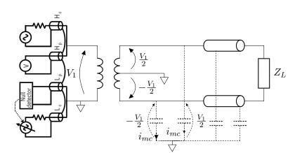
Figure 2.13 – Common-mode analysis of balun-isolated measurement
