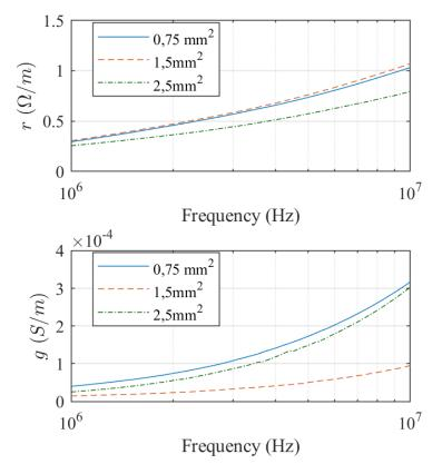
Figure C.7 – Two-conductor cables loss related parameters
