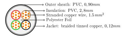
Figure 5.5 – Cross-section of the  $4x1, 5\,mm^2$  cables
