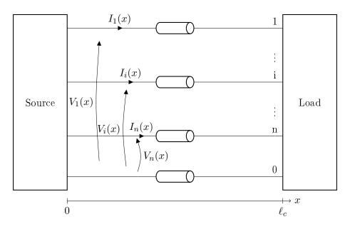
Figure 3.1 – Multiconductor transmission line, variables definition
