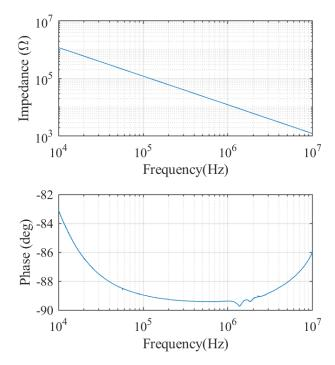
Figure 2.21 – Voltage probe input impedance
