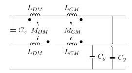
Figure 5.34 – Filter structure
