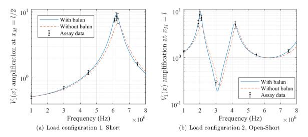
Figure 3.13 – Experimental validation : resonance-due voltage amplification
