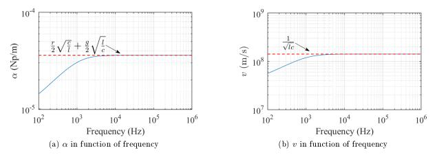
Figure 2.5 –  $\gamma = \alpha + j \frac{\omega}{v}$  in function of frequency
