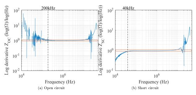
Figure E.4 – Logarithmic derivative of the measured input impedance of the cable, the lowest frequency to which they can be considered constant is marked with dotted line
