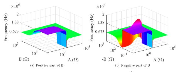
Figure C.9 – First resonance frequencies of the two-conductor  $2.5 mm^2$  cable of length 50 m, in function of the load
