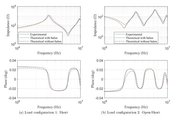
Figure 3.16 – Experimental validation : input impedance
