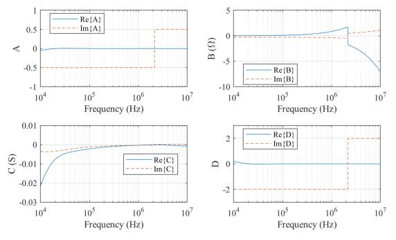
Figure E.2 – ABCD parameters of the Minicircuits T6-4T balun
