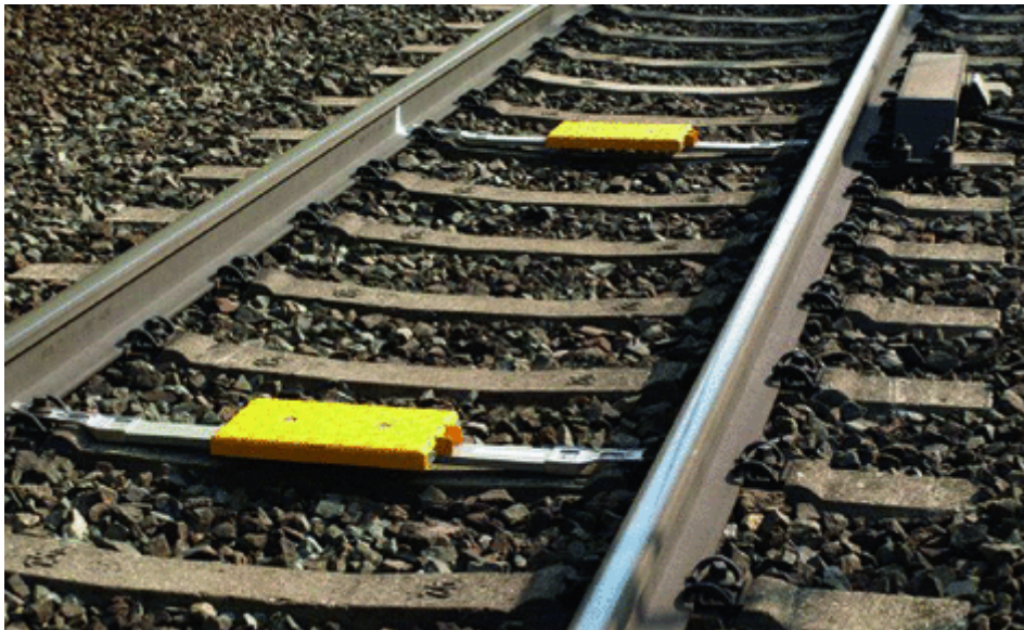
Figure 2-4 Balise between the rails (and its LEU)*
