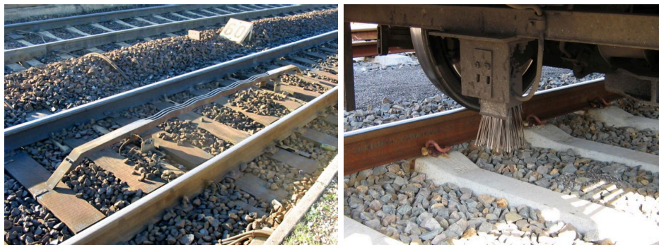
(a) (b) Figure 2-7 Trackside and onboard device of BRS ( Crocodile ) system*
