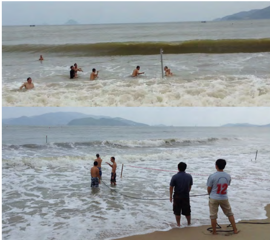
Figure 4.8: An example of how to deploy the Bathymeter. In the upper picture shows to take Bathymeter out of the surf zone, then drag shoreward to get the entire profile in lower picture
