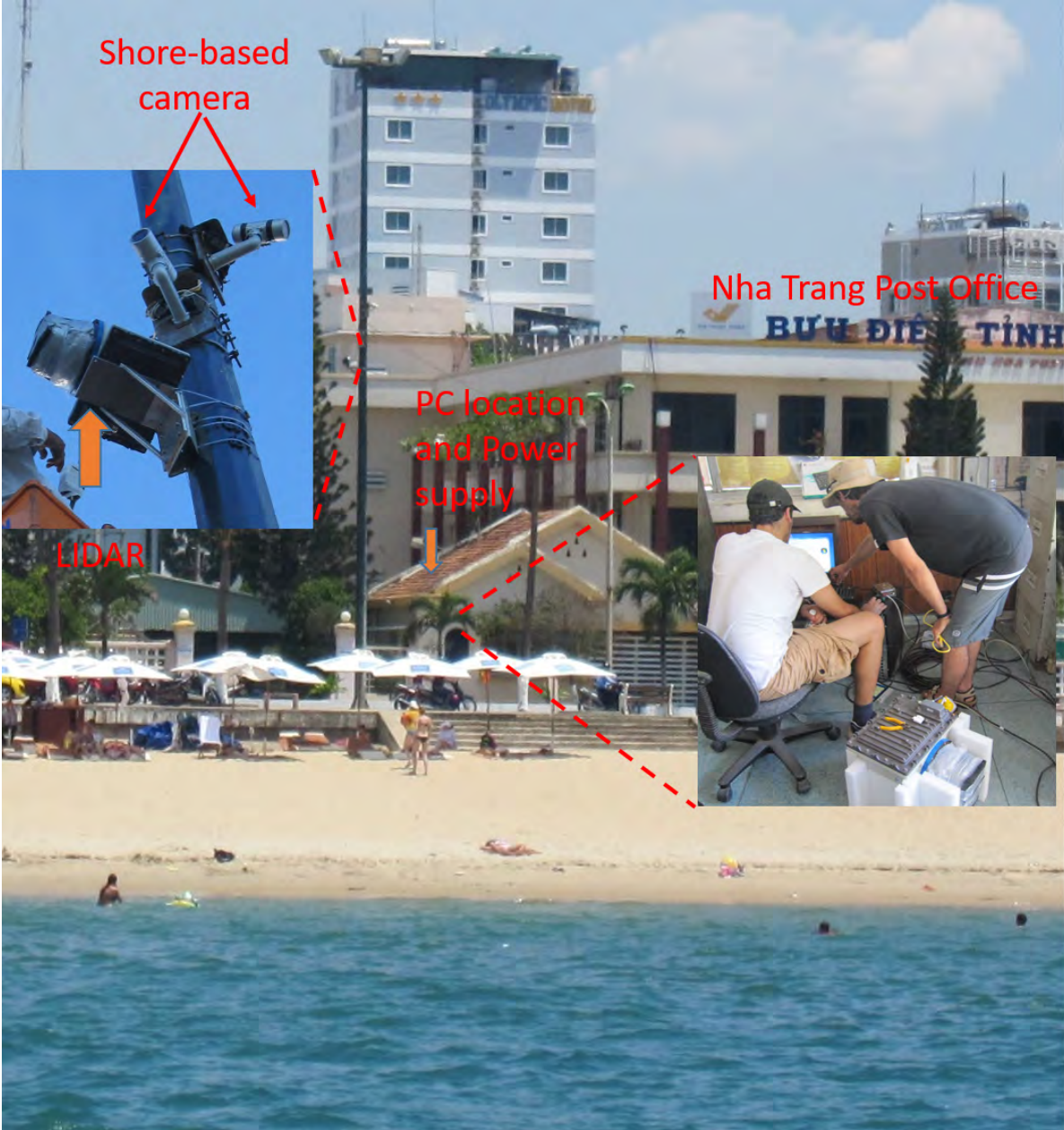
Figure 4.13: Field photo showing the setting of a long-term LIDAR station at Nha Trang beach.
