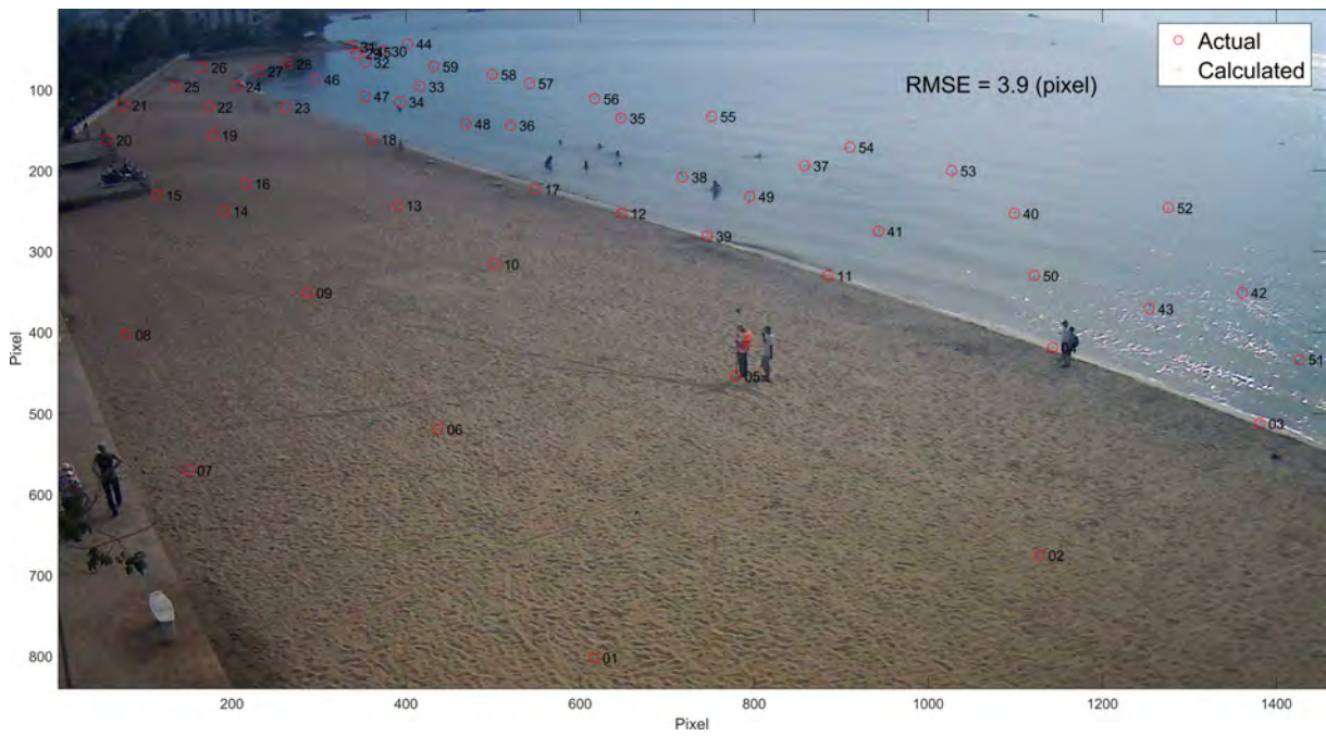
Figure 3.5: Camera calibration results of NNT camera, applying field calibrations using 59 in situ GCPs. The actual pixel coordinates (open red circle) of the object are determined manually. The pixel coordinates (red cross) were projected using georeference calibration parameters in Table 3.1.
