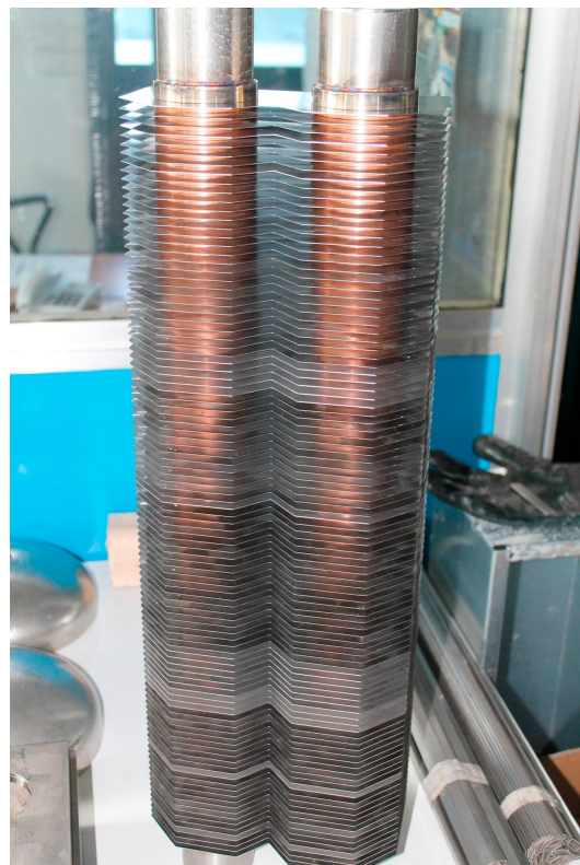
Figure 2.2: A picture of the twin columns of the PROGEO reactor.[137]
