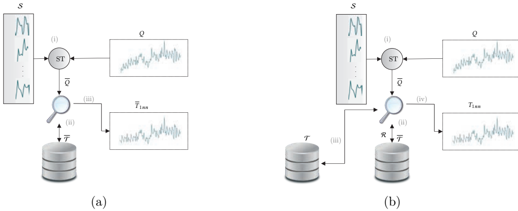
FIGURE 3.2 – Diagram illustrating the difference between methods directly (a) and refined (b). In (a), the retrieval starts by transforming the query Q to \bar{Q} using the dictionary \mathcal{S} ; then using \bar{Q} , we search for the closest entry in \bar{\mathcal{T}} (ii); finally the closest element \bar{T}_{1nn} is returned (iii). In (b), after transforming Q in \bar{Q} (i), the search initially returns the set \mathcal{R} of the closest elements (ii); then, a refinement is done by comparing Q and the entries in \mathcal{R} using the DTW (iii); finally, the closest element is returned (iv).
