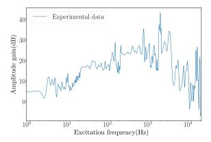
Fig. 8. Amplification (in dB) is plotted as function of the frequency at which a piezoelectric transducer excites the membrane. Amplification was derived from the difference of amplitude between the transducer vibrating alone and its action as it was put on the balloon. For convenience, a sweep of frequencies was performed. The distance to the microphone remains constant between the two sound samples.
