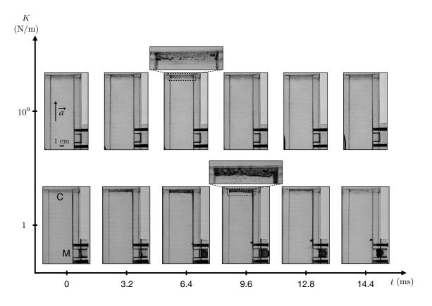
Figure 2.3: Chronophotographies of the impact of the reservoir on a damper for different values of the bending stiffness K of the membrane. The shock results in a vertical maximal acceleration  $a \approx 150$  g applied on the container for a time  $\sim 7$  ms. The contrecoup region C is located at the point opposite of impact.
