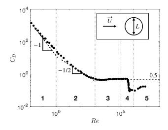
Figure 2: Experimental measurements of the drag coefficient  $C_D$  of a sphere of diameter L as a function of the Reynolds number  $Re = UL/\nu$ . In this expression, U is the flow velocity and  $\nu$  the kinematic viscosity of the fluid. Five characteristics regimes are identified in this curve. Figure reproduced from [1].
