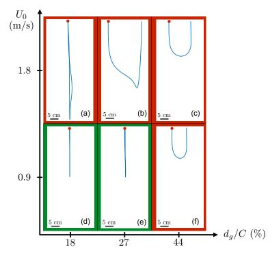
Figure 8.8: Trajectories of the center of mass of the projectile calculated from the numerical resolution of the equations of motion at different values of the impacting velocity  $(U_0)$ , and for different positions of center of gravity of the projectile  $(d_g/C)$ . A trajectory is considered unstable if we have  $\frac{d\theta}{dt}(t=0^+) > 0$ . Stable trajectories are boxed in green, unstable ones in red.
