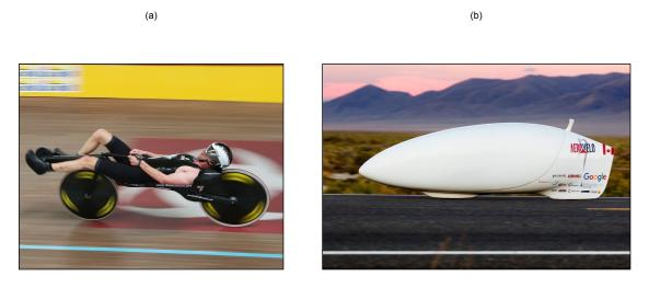
Figure 4: (a) Picture of Aurélien Bonneteau for his attempt to beat the hour record on track in 2012. He managed to bike 56.7 km in an hour. The peak record for a 200 m section on a similar bike is 74 km/h. (b) Picture of the fully faired bike used to break the record of velocity on a 200 m section in 2016. The velocity reached was 144.2 km/h on a slightly downhill section (-0.6 % slope).
