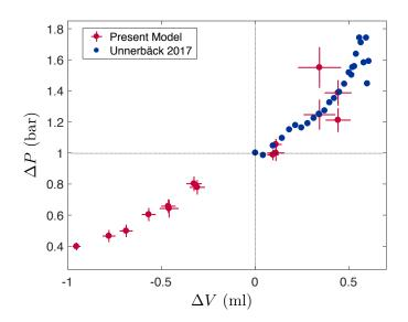
Figure 2.4: Relationship between the pressure and volume variations  $\Delta P$  and  $\Delta V$ , for a human head (blue data) and for our model system (red data). Both series of data overlap if we use a soft flexible membrane of bending stiffness 1 N/m. Human data are taken from Unnerbäck 2017 where peak values have been discarded. Pressure in our set-up are measured for a membrane of thickness 3.5 mm an then extrapolated for the equivalent membrane of thickness 1 mm.
