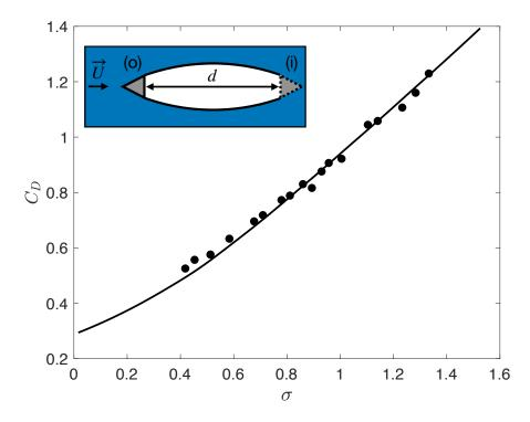
Figure 9: Drag coefficient of a 30° wedge as a function of the cavitation number  $\sigma$ . Figure adapted from [12]. Experimental data are corrected to account for the finite width of the test section. Solid line is the Riabouchinsky model [10]. Inset: sketched of the Riabouchinsky model. The closing of the cavity is imposed on a image (i) of the wedge placed at a distance d downstream the object (o).
