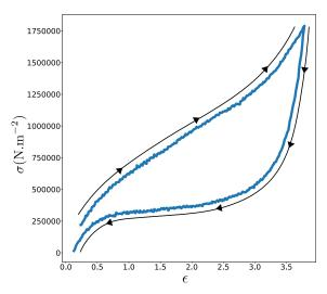
Fig. 6. Traction curve of an elastic rubber balloon. The stress  $\sigma$  is plotted as a function of the relative elongation of the band  $\epsilon$ . Black arrows show the path of the deformation. Their is a non-linear stretching deformation (arrows upwards). The loosening (arrows downwards) does not follow the initial curve, a characteristic feature of the plastic domain.
