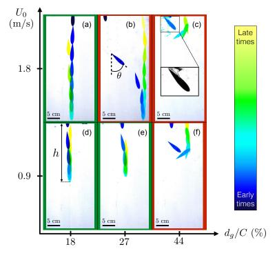
Figure 8.1: Chronophotographies of the projectile trajectories for various impacting velocities  $U_0$ , and for various distances  $d_g$  between the center of gravity of the projectile and its leading edge. The center of buoyancy is located at 37.5 % of the total chord from the leading edge. For all chronophotographies, frames are separated by 0.15 seconds. The stable trajectories are boxed in green whereas the unstable ones are boxed in red.
