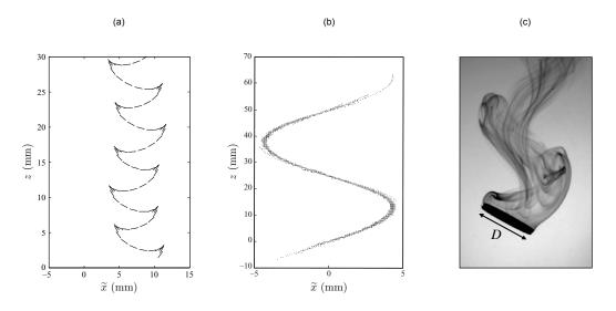
Figure 7.3: (a) Experimental fluttering of a plate of thickness 0.089 cm and of aspect ratio 1/14 at a Reynolds number Re = 1147. The time step is 0.04 s. Figure taken from [124]. (b) Trajectories, in the mean oscillation plane  $(z,\tilde{x})$ , of 71 rising bubbles of radius 2.5 mm. Figure taken from [125]. (c) Smoke visualization of the wake behind a disk of aspect ratio 1/10 at  $Re \approx 240$ . Picture adapted from [126].
