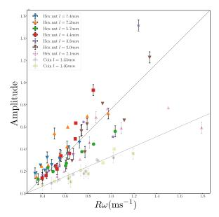
**Fig. 9.** The amplitude A plotted as a function of  $R\omega$  for the same type of nuts, same rotation speeds and same balloon radii as above. Linear regressions are plotted for each type of nuts. Coin data points are plotted with low opacity due to deviation from the regression coefficient of the hex nuts.
