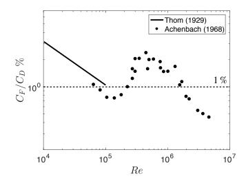
Figure 3: Contribution of the skin friction to the total drag  $(C_F/C_D)$  as a function of the Reynolds number. Figure reproduced from [2]. Dot are experimental data corrected to account for the finite width of the tunnel. Solid line is a semi-theoretical prediction in the sub-critical regime drawn from [3].
