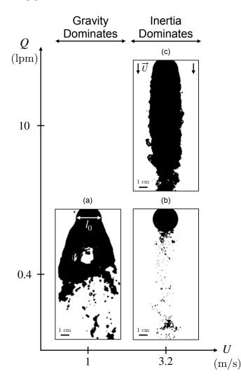
Figure 6.1: Pictures of the structures obtained when injecting air at the back of a sphere, depending on the air injection rate Q and the flow velocity U. Flow is running downward and the sphere of diameter 3 cm is always at the top of the picture. For a flow velocity of 1 m/s and Q > 2 lpm, the tunnel is blocked due to the large width of the bubble and stops running.
