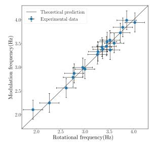
**Fig. 5.** Amplitude modulation frequency plotted against the macroscopic rotational frequency of the nut. The frequency was averaged over a period of 10 modulations for each experiment. The macroscopic rotational frequency was derived from videos of the balloon taken at 30 fps, using a regular camera.
