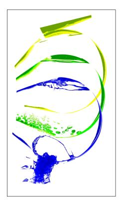
Chronophotography of the shattering of a rounded bottom flask induced by the collapse of cavitation bubbles in the region opposite to the point of impact. Yellow is for t = 0 (i.e. impact of the hammer), green is for t = 1.2 ms and blue for t = 6.65 ms.
