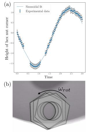
Fig. 4. (a) Experimental data of the height of a corner of the nut during one rotation of the nut extracted using Tracker (soft-ware). A sinusoidal fit is performed on the experimental data and plotted in solid line. (b) Superposition of three images of the nut rolling on the membrane taken with a high-speed camera at 3000 fps. For visualisation purposes the hex nut is redrawn.
