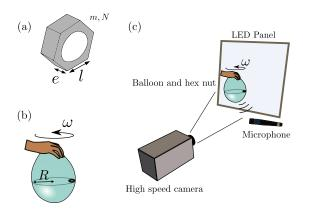
Fig. 1. Experimental setup and nomenclature. (a) Sketch of the hex nuts used in experiments. A nut is characterised by its number of sides N, it's side length l, its width e and its mass m, (b) Close sketch of the balloon, characterised by its radius R and its rotating speed  $\omega$ . (c) Sketch of the experimental setup.
