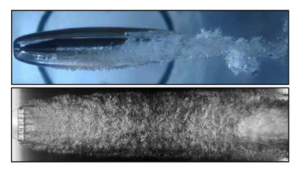
Ventilated cavities behind a disk (top picture) and a fence (bottom picture).
