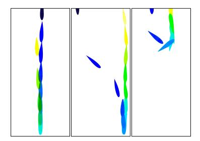
$Chronophotography\ of\ three\ different\ underwater\ trajectories\ of\ floating\ streamlined\ projectile.$
