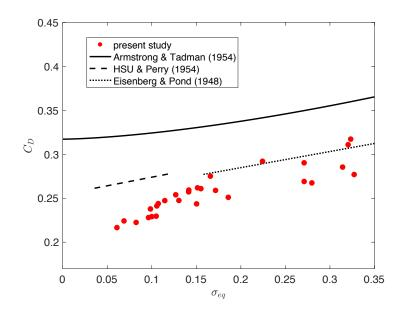
Figure 6.7: Drag coefficient  $C_D$  of a sphere as a function of the equivalent cavitation number  $\sigma_{eq}$ .  $\sigma_{eq}$  is evaluated using our measured cavity length and [88]. Theoretical work of [89] is plotted in solid line. Mean line for experimental results [90, 91] are drawn in dashed and dotted lines.
