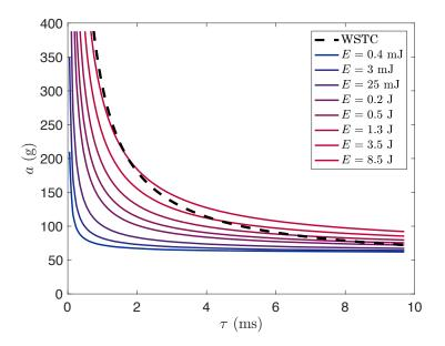
Figure 3.6: Iso-energy curves in the  $(a, \tau)$  diagram and comparison with the Wayne State University Curve. The energy  $E = \rho a L R_{max}^3$  released by a bubble is calculated using equation (3.15), which allows us to plot iso-energy curves in the  $(a, \tau)$  diagram. Varying E between 0.4 mJ and 8.5 J generates a family of curves that gradually evolve towards the WSTC (dashes) as E increases. The value at which they match is  $E_D=8.5$  J.
