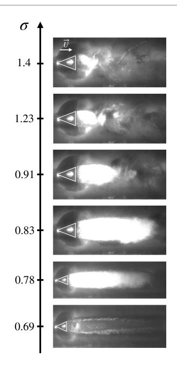
Figure 8: Picture of a 45° angle wedge and its wake in a cavitation tunnel for various cavitation numbers. Figure adapted from [8]. Cavitation number is  $\sigma = (p_{\infty} - P_{vap})/1/2\rho U^2$ , where  $p_{\infty}$  is the pressure far from the projectile,  $P_{vap}$  the vapor pressure of water,  $\rho$  its density and U the velocity of the flow. The base of the cavitator is 2 cm. The shutter speed is below 1/50000 s.
