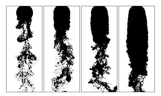
Pictures of a sphere with air injected at its back at an increasing rate from the left to the right picture.
