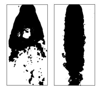
Two illustrations of the ventilated cavities behind a sphere that can be obtained with the experimental set-up presented in this chapter.
