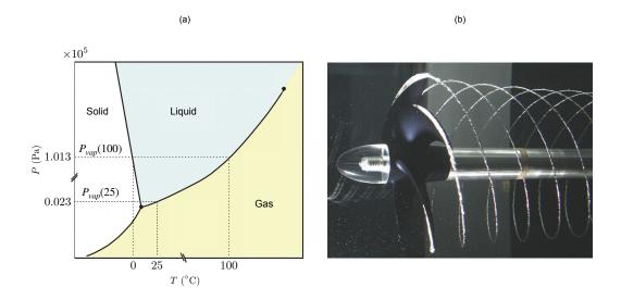
Figure 7: (a) Phase diagram of water as a function of its temperature T and its pressure P. The vapor pressure of water is written  $P_{vap}$ . (b) Picture of the cavitation trail observed behind a ship propeller at the Cavitation Research Laboratory of the Australian Maritime College (http://www.amc.edu.au/facilities/cavitation).
