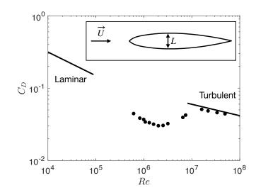
Figure 5: Drag coefficient  $C_D$  of a streamlined body of revolution as a function of the Reynolds number  $Re = UL/\nu$ . Figure reproduced from [1]. Solid lines indicate the trends for sub and super critical regimes. Dots are experimental data. The profile of the projectile used is the one of the R101 airship and is sketched in the inset. Drag coefficient is based on frontal area.
