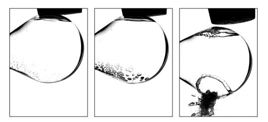
Fluid container accelerated when hit by a hammer: Cavitation bubbles grow in the region opposite of the point of impact and shatter the reservoir.
