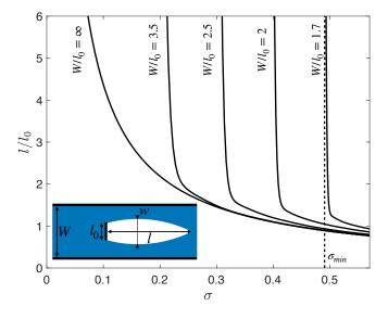
Figure 4.3: Numerical simulations of the dimensionless length of the cavity  $l/l_0$  as a function of the cavitation number  $\sigma$  for different blockage ratio  $\mathcal{B} = W/l_0$  (see inset). Figure adapted from [6].
