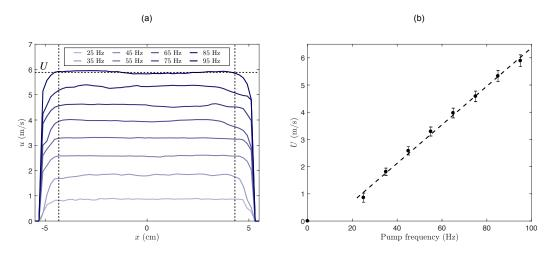
Figure 5.3: (a) Cross-stream profiles of the streamwise velocity u for running frequencies of the pump ranging from 25 Hz to 95 Hz. Walls of the tunnel are located in  $x = \pm 5.5$  cm. (b) Average streamwise velocity U in the center part of the the tunnel as a function of the pump frequency. Dotted line is an affine fit in the range of accessible running frequencies (25 to 100 Hz).
