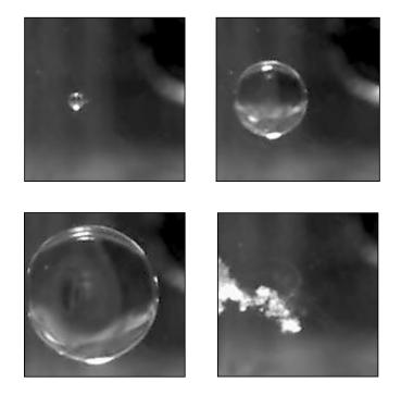
Illustration of the growth and the collapse of a bubble recorded using the experimental set-up described in this chapter.
