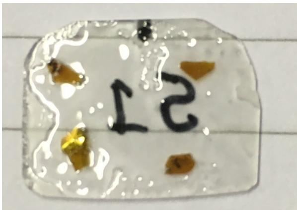
FIGURE 6.19. Photographic image of four samples prepared and attached to a sapphire crystal.
