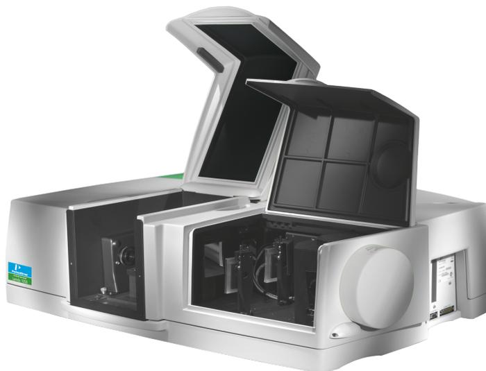
FIGURE 4.4. Perkin Elmer Lambda 950 spectrophotometer image taken from the Perkin Elmer website.
