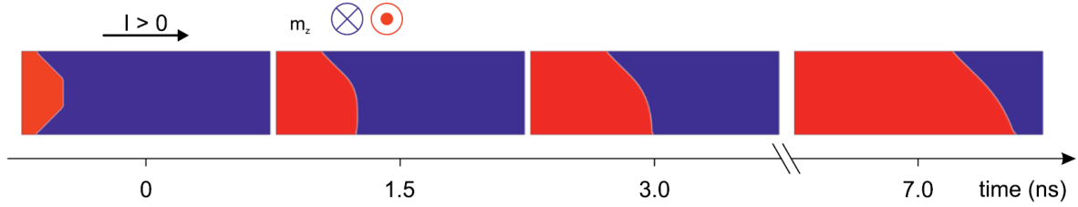
Figure IV.3 Snapshots from micromagnetic simulations of the arc-shaped DW_{U-D} driven by electric current. The current density is 4.5 \cdot 10^{12} \text{ A.m}^{-2} . The wire is 4.5\text{-}\mu\text{m} -length and 1.5\text{-}\mu\text{m} -width. After \approx 1.5 \text{ ns} , the fastest DW is expelled from the wire. The final tilt angle corresponds to the DW slowest front and is in agreement with previous studies of the Pt/Co structures. Extracted from [Baumgartner and Gambardella, 2018].
