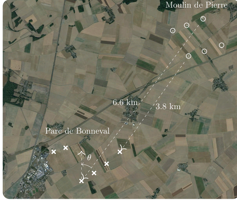
Figure 4.1 | Satellite image of Parc de Bonneval and Moulin de Pierre extracted from Google Earth. The white crosses display the turbine location at Parc de Bonneval and the white circle at Moulin de Pierre location. Typical distances and angle between the two farms are also shown.
