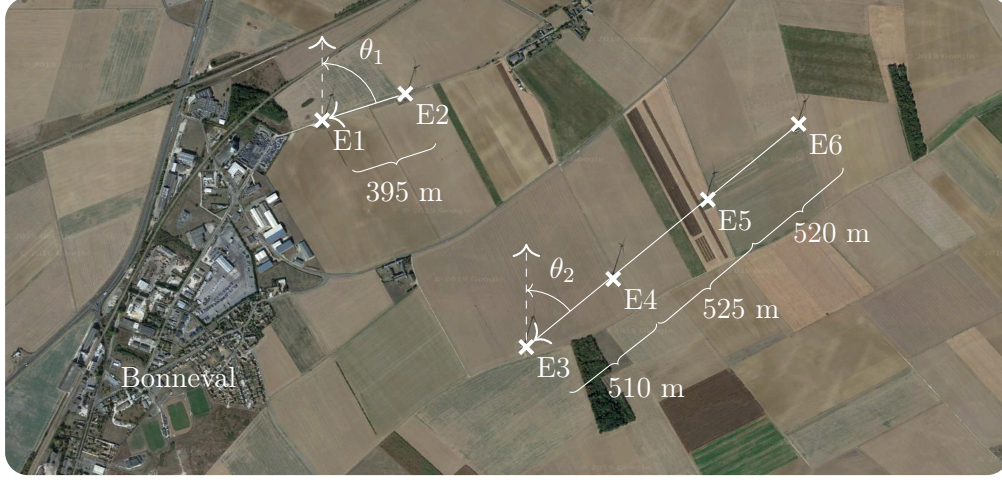
Figure 3.5 | Satellite image of Parc de Bonneval extracted from Google Earth. The white crosses display the turbine location with their respective number. Two lines are visible. One between E1 and E2 (the angle formed between E1-E2 and the south-north direction is denoted \theta_1 ). The second line is formed by the turbines 3, 4, 5 and 6 (the angle between these turbines and the south-north direction is denoted \theta_2 ). The distance between the turbines is added.
