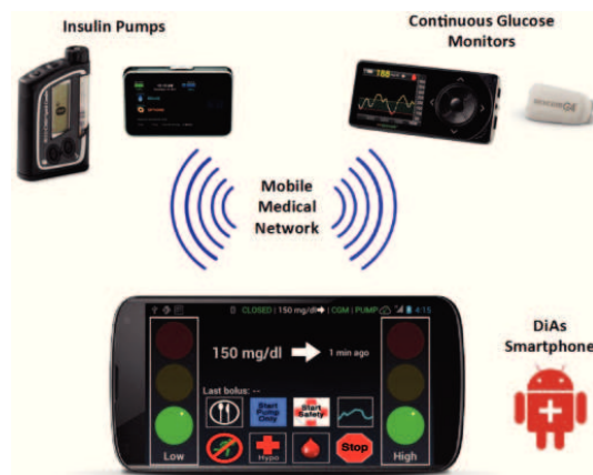
Figure 2.5 A smart-phone based portable artificial pancreas: Diabetes Assistant system (Dias) as presented in [28] where it was used in clinical trials.
