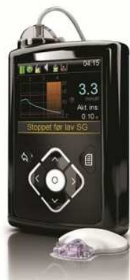
Figure 2.4 Insulin delivery system MiniMed ® 640G system ^ , insulin pump in black and a CGM in white.
