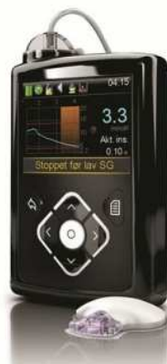
Figure 2.4 Insulin delivery system MiniMed ® 640G system ^ , insulin pump in black and a CGM in white.
