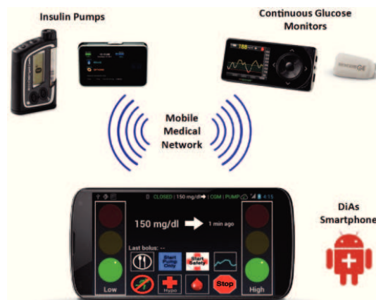
Figure 2.5 A smart-phone based portable artificial pancreas: Diabetes Assistant system (Dias) as presented in [28] where it was used in clinical trials.
