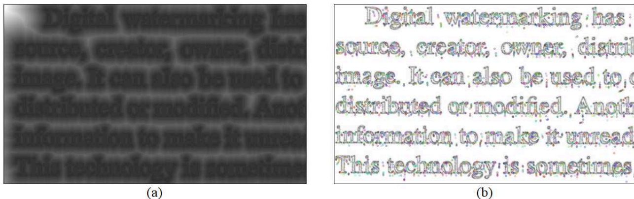
Figure 3.13: Detection of feature points: The distance transform document (a) and extracted feature points (b).
