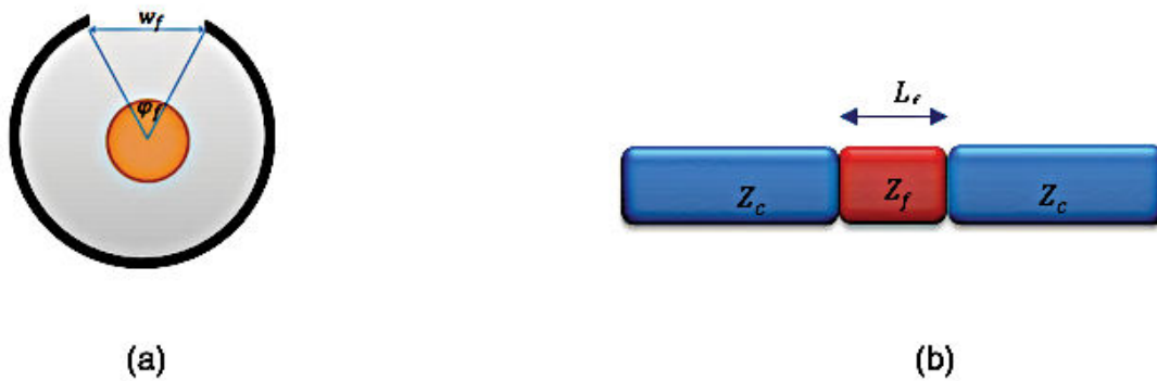
Figure 1-18. Scheme of a chafed cable.
