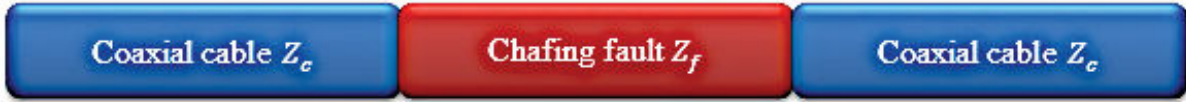
Figure 1-15. Modeling of a damaged coaxial cable called the chafe model with Z_f is the fault's impedance.
