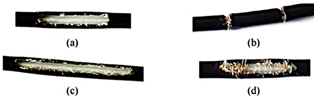
Figure 5-16. Different types of soft faults: (a) 2.5-cm-long 90^\circ cut in the insulator and shield of the coaxial, (b) cuts in the shield and insulator, (c) 4-cm-long 90^\circ cut in the insulator and shield of the coaxial, and (d) 2-cm-long <30^\circ long cut on the insulator and shield of the coaxial.
