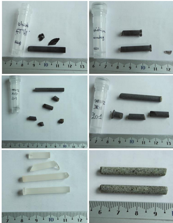
Figure B.46 Cores samples realized with the drilling machine at the LMV. Core samples of ATHO, Güney Dag, DR07-201, DR11-201, Haplobasalt and RP4 peridotite (from to left to bottom right respectively).
