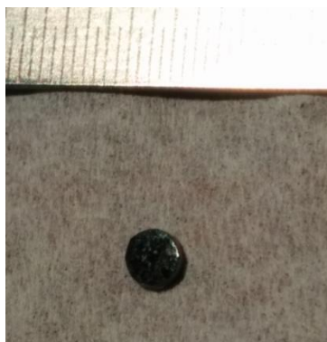
Figure III.10 Photograph of the synthesis products after double polishing. Sample was then inserted in the EC/SV experiments.
