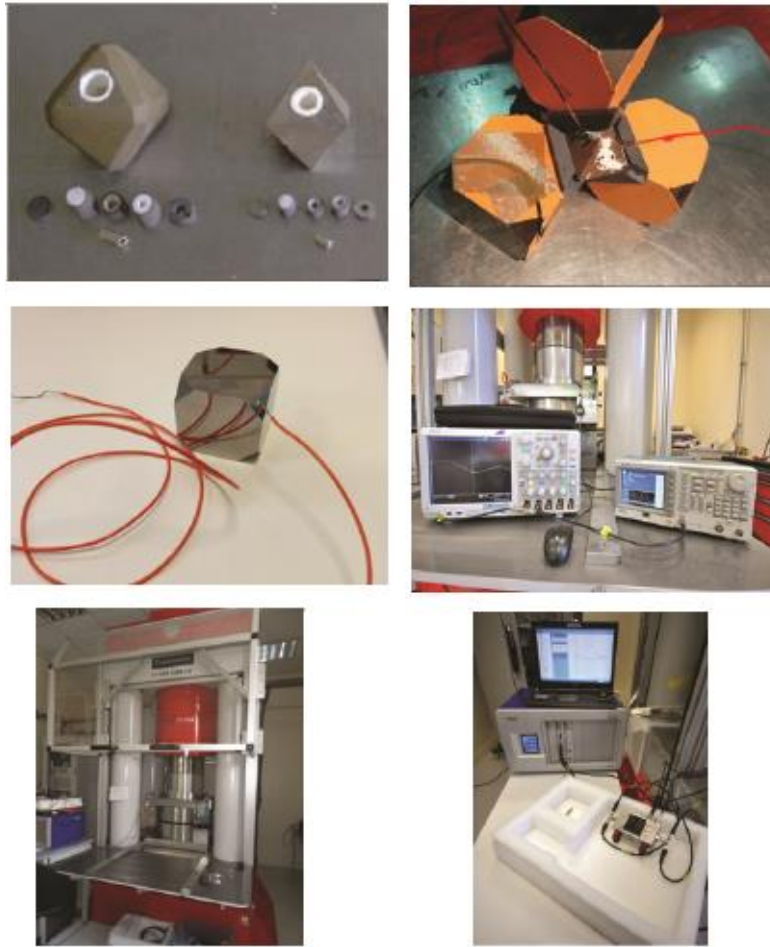
Figure III.12 Photographs illustrating the preparation of high pressure and high temperature experiments and their realization. From top left to bottom right: a) experimental assemblies (25/17 and 18/11) used for this study with graphite heater and rhenium capsules. b) Assemblage of octahedron on the cubes. One can remark the specific geometry required for the thermocouple and electrode wires which is unique for this experiment given that the position in the primary anvils guide block is fixed for the transducer. c) Boston Piezoelectric LiNbO 3 transducer fixed (tin solder) at the polished corner of 11 mm truncation anvil. d) Tektronix digital phosphor oscilloscope (left) and Tektronix AFG3101C wave function generator (right) used for sound velocity generation and record. e) 1500 Ton (Voggenreiter Mavo press) multi-anvil apparatus used at the Laboratoire Magmas et Volcans. f) Solartron ModuLab MTS Impedance/Gain-phase analyzer used to measure electrical conductivity. For scale octahedron side length is 24 and 18 mm (a), 18 mm (b), truncation corner 11 mm (c), computer mouse at foreground (d), Multi-anvil apparatus is 3.2 m high (e), 15" laptop (f).
