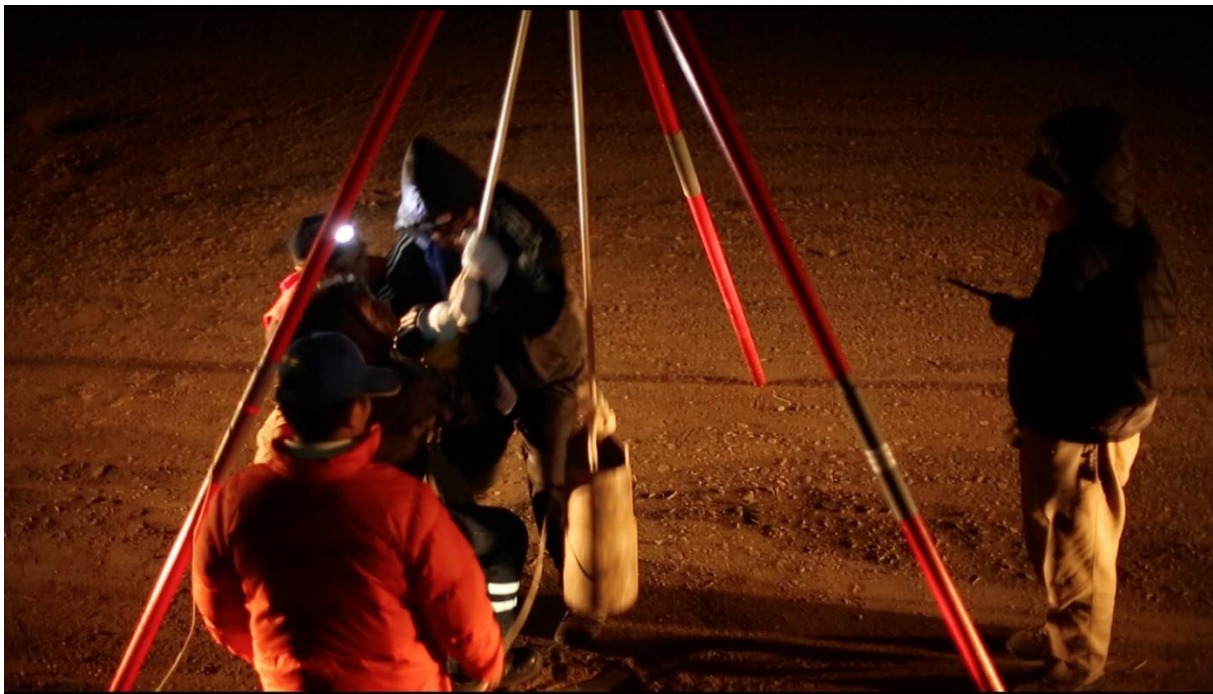
Figure S 6-11 Estimation of the P wave velocities in the Maca landslide. Picture of the source system. An 80-kg mass was pulled up to approximately 2 m high using a tripod and a pulley and dropped onto a metallic plate. Data were acquired at night to diminish the impact of wind and anthropogenic noise (mainly coming from a road attracting considerable tourist traffic) on the signal recorded. Picture by Larose E.
