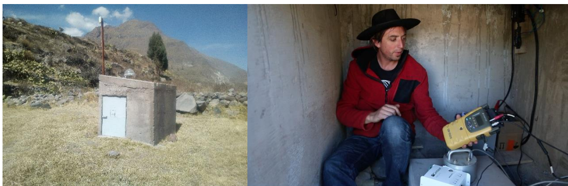
Figure S 6-2 a, Picture of the hut containing the GPS and the seismic station. The antenna of the GPS is visible on the top of the hut. b, interior of the hut, with the GPS and the seismometer installation displayed.
