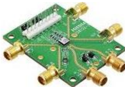
Figure III.7: Circuit T&HA 'Hittite HMC760LC4B'.
