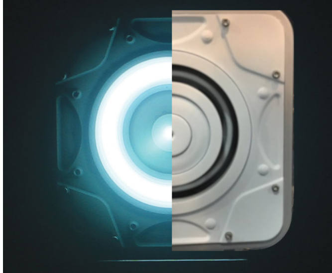
FIGURE 1.4 – Front view of an HET, the BHT-1500 from Busek, USA, switched on (left) and off (right). The cathode is located at the center.
