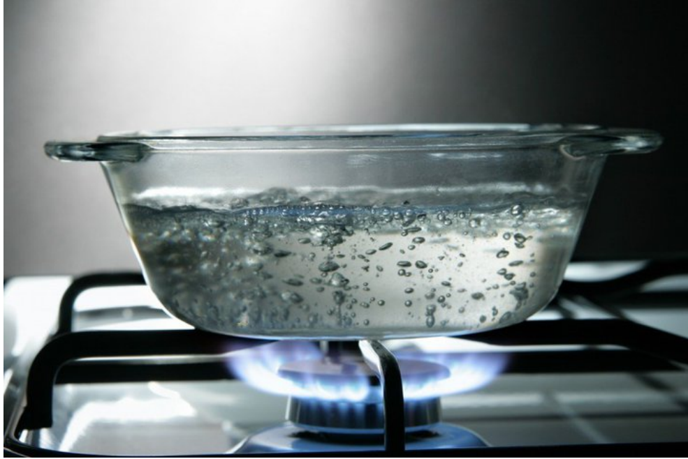
Fig. 1.1 – Nucleate boiling in a heated tureen. Credit: Roman Sigaev/Fotolia.
