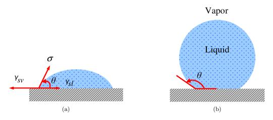
Fig. A.5 – Surface wettability : (a) wetted or hydrophilic surface ( $\theta < \pi/2$ ), (b) unwetted or hydrophobic surface ( $\theta \ge \pi/2$ ).
