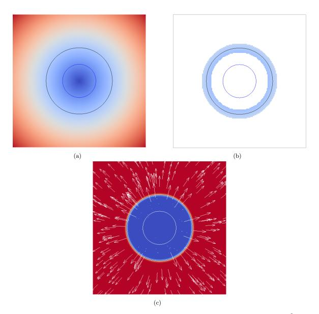
Fig. 5.6 – Interface location at final time on the finest structured grid considered ( $\Delta x = 5 \times 10^{-5}$  m) for (a) Case 1, (b) Case 2 and (c) Case 3. The initial interface is represented in blue (in white on (c)), the computed interface at final time, in black. Our FMM implementation reinitializes  $\phi$  only in the narrow band around the interface to save computational time. The liquid and vapor velocity fields are represented on (c).
