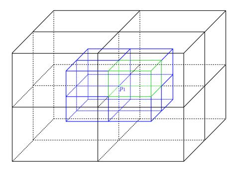
Fig. 3.4 – Total control volume of node  $\mathbf{p}_1$ . Each contribution is built according to the method illustrated in Figs. 3.2 and 3.3. The contribution shown in Fig. 3.2 is represented in green.
