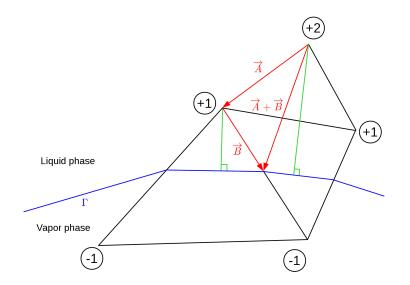
Fig. 3.11 – Computation on a node of band level 2 of the signed distance function  $\phi$  to the interface  $\Gamma$  by Eq. (3.26) where the vector summation is done on the grid edges shown in red. The resulting  $\phi$  value is equal to the norm of vector  $\mathbf{A} + \mathbf{B}$ . The exact value is given by the length of the green segment.
