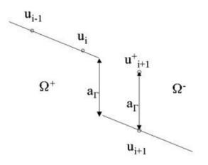
Fig. 2.5 – Illustration of the Ghost Fluid Method in one dimension where the interface  $\Gamma$  separating subdomains  $\Omega^+$  and  $\Omega^-$  is located between nodes *i* and *i* + 1. The physical field *u* is extrapolated across the interface from node *i* to node *i* + 1, where the ghost value is noted  $u_{i+1}^+$ , artificially removing the discontinuity  $a_{\Gamma}$  of *u* at the interface.
