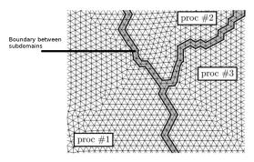
Fig. 3.6 – MPI parallelism using the Simple Domain Decomposition method. Each core has knowledge of only one subdomain.
