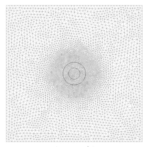
Fig. 6.9 – Coarsest unstructured grid ( $\Delta = 1.875 \times 10^{-4} \,\mathrm{m}$ ) used to perform the test case in two dimensions presented in Section 6.6.1.2. The grid is refined in the area in which the interface will evolve. The small circle represents the initial interface location of radius  $R_0 = 1 \times 10^{-3} \,\mathrm{m}$ , the bigger circle represents the final theoretical interface location (the radius is twice the initial one).
