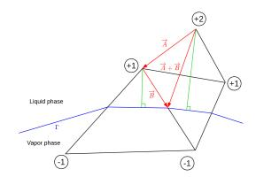
(b) Computation of signed distance values on neighbor nodes of the closest nodes to the interface (band level +2).
