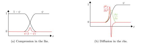
Fig. 2.4 – The compression and diffusion effects in the reinitialization equation of the Conservative Level Set function proposed by Olsson et al. [58, 59].
