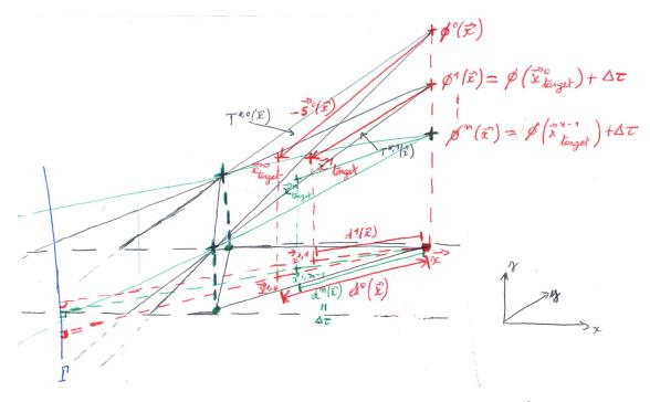
Fig. E.11 – For each iteration *n*, the distance between node **x** and point  $\mathbf{x}_{\text{target}}^{n-1}$  is equal to  $\Delta \tau$ . After the last iteration *N*, one has  $\nabla \left( \phi |_{T^*(\mathbf{x})} \right) = \mathbf{n}_{\Gamma}(\mathbf{x})$ , i.e. the tilt direction of the final plane  $P^N$  is equal to  $\mathbf{n}_{\Gamma}(\mathbf{x})$ , and one has  $\phi^N(\mathbf{x}) = \phi^{N-1}(\mathbf{x}_{\text{target}}^{N-1}) + \Delta \tau$  by Eq. (E.22).
