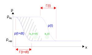
(b) Advection of diffuse interface with phase change : the interface motion is faster than the fluid particle motion due to the source term in Eq. (1.17). As a result, the fluid particle exits the interface region. The hatched area represents the contribution of phase change to the interface motion.
