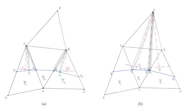
Fig. F.2 – Reinitialization of the signed distance function by the GMM on (a) nodes of band level 1, and (b) nodes of band level 2.
