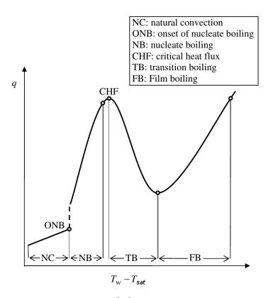
Fig. A.7 – Pool boiling curve of Nukiyama [56] representing the imposed heat flux q at the wall with respect to the wall superheat  $T_w - T_{\text{sat}}$  [31].
