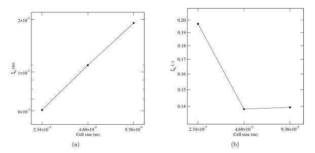
Fig. 6.8 - Error on (a) the final *x*-component of the interface normal vector and relative error on (b) the final interface curvature for the two-dimensional simulations on equilateral triangles presented in Section 6.6.1.1.
