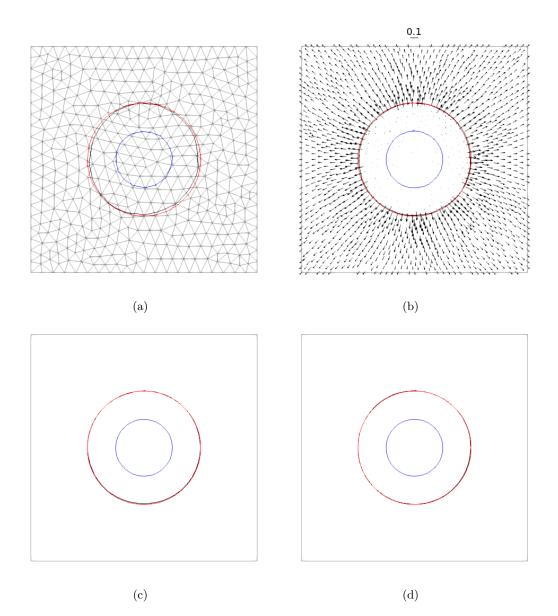
Fig. 5.11 – The results for the Case 7 on four different unstructured grids are plotted at final time with a characteristic cell size of (a)  $4 \times 10^{-4}$  m, (b)  $2 \times 10^{-4}$  m, (c)  $1 \times 10^{-4}$  m and (d)  $5 \times 10^{-5}$  m. The initial interface is plotted in blue, the computed interface in black, and the theoretical interface in red. For clarity, only the coarsest grid is represented in (a). The computed liquid and vapor velocity fields are plotted in (b).
