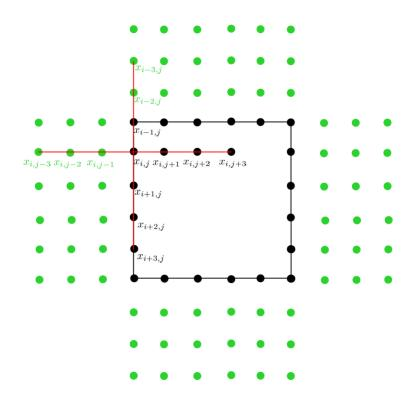
Fig. 5.5 – Addition of a ghost domain (in green) to the initial domain (in black) in order to build neighbor lists composed of three neighbors on top, right, bottom and left of all nodes located on and close to the initial domain boundaries.
