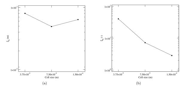
Fig. 6.15 – Error on (a) the final *x*-component of the interface normal vector and relative error on (b) the final interface curvature for the three-dimensional simulations on unstructured grids presented in Section 6.6.2 with a Jakob number of 5.
