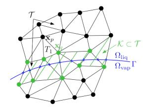
Fig. E.2 – Notations of Alg. 2 :  $\mathcal{T}$  is the simplicial grid,  $\mathcal{K} \subset \mathcal{T}$  is the simplicial subset of  $\mathcal{T}$  intersecting the interface  $\Gamma$ ,  $T_1 \in \mathcal{T}$  is a simplex, nodes  $\mathbf{x}_p$  and  $\mathbf{x}_q$  are summits of  $T_1$ , and  $\Omega_{\text{liq}}$  is the region occupied by the liquid phase. As opposed to node  $\mathbf{x}_p$ , node  $\mathbf{x}_q$  belongs to simplices of  $\mathcal{K}$ .
