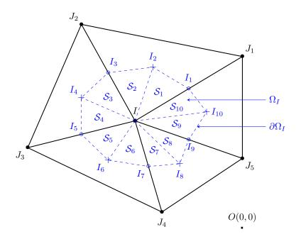
Fig. 6.3 – The control volume  $\Omega_I$  associated to node  $\mathbf{x}_I$  represented by point I is the disjoint union of simplices  $S_1, \ldots, S_{10}$ . The symbol  $\bullet$  denotes the grid nodes I and  $J_1, \ldots, J_5$ , +, the grid element barycenters  $I_2$ ,  $I_4$ ,  $I_6$ ,  $I_8$ ,  $I_{10}$ ,  $\circ$ , the grid edge midpoints  $I_3$ ,  $I_5$ ,  $I_7$ ,  $I_9$ , and  $\bullet$ , the point O (frame origin) which does not necessarily represent a grid node.
