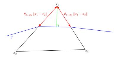
Fig. 3.10 – Computation on node  $\mathbf{x}_1$  (band level 1) of the signed distance function  $\phi$  to the interface  $\Gamma$  by Eq. (3.25) where the relative distance  $\theta_{\mathbf{x}_1,\mathbf{x}_2}$  is given by Eq. (3.24). The exact value of  $\phi(\mathbf{x}_1)$  is given by the length of the green segment.
