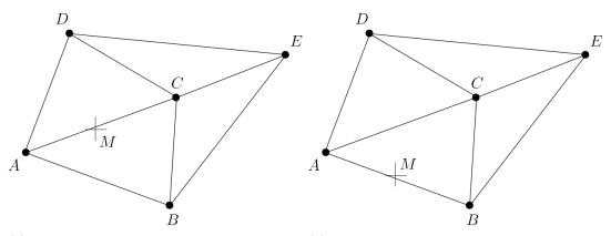
(a) Point M is close to edge AC, directly related (b) Point M is close to edge AB, not directly to node  $\mathbf{x}_C$ .
