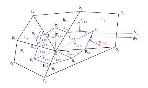
Fig. 3.1 – Example of a two-dimensional control volume used in the Finite Volume Method. The control volume associated to node  $\mathbf{p}_1$  is defined by the neighbor grid element barycenters and edge midpoints.
