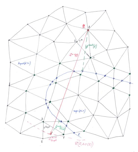
Fig. E.7 – In this example, the pseudo-time step  $\Delta \tau(\mathbf{x})$  is node-dependent. The shoot vector  $\mathbf{s}^{n-1}(\mathbf{x})$  is almost collinear to the interface normal vector  $\mathbf{n}_{\Gamma}(\mathbf{x})$  but crosses the interface. Proposition P is true but Eq. (E.22) fails to update  $\phi^n(\mathbf{x})$  accurately.
