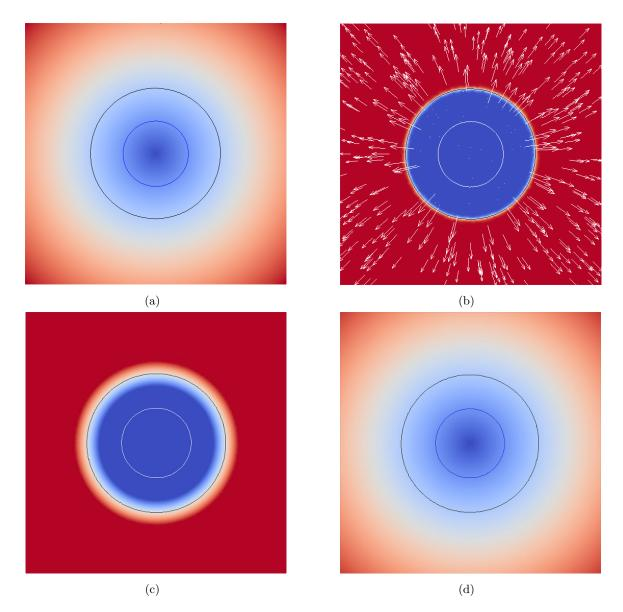
Fig. 5.8 – Interface location at final time on the finest unstructured grid considered ( $\Delta x = 5 \times 10^{-5} \,\mathrm{m}$ ) for (a) Case 4, (b) Case 5, (c) Case 6 and (d) Case 7. The initial interface is represented in blue on (a) and (d) and in white on (b) and (c), the computed interface at final time, in black. The liquid and vapor velocity fields are represented on (b).
