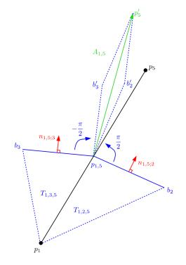
Fig. 3.5 – Definition and storage of vector  $\mathbf{A}_{1,5}$  at edge  $(\mathbf{p}_1, \mathbf{p}_5)$  as the sum of the oriented surfaces  $\|\mathbf{b}_3 - \mathbf{p}_{1,5}\| \mathbf{n}_{1,5;3}$  and  $\|\mathbf{b}_2 - \mathbf{p}_{1,5}\| \mathbf{n}_{1,5;2}$ .
