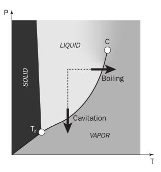
Fig. 1.2 – Pressure-temperature (P-T) phase diagram for water adapted from the book of Franc and Michel [23]. The triple point  $T_r$  is the point at which the three phases coexist, the critical point C separates the liquid and vapor domains.
