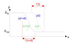
(a) Advection of diffuse interface without phase change. The fluid particle centered at point  $\mathbf{x}_P$  is at rest with respect to the interface frame.
