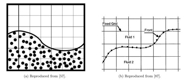
Fig. 2.2 – Front Tracking Methods : (a) in the MAC method of Harlow and Welch [32], markers are distributed in all the phase of interest and the interface is defined as the border of the area filled with markers ; (b) Tryggvason et al. [89, 41, 87] adapted the MAC method with markers distributed only at the interface, leading to *the* Front Tracking Method.
