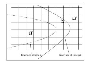
Fig. 6.1 – The node with a question mark is swept over by the interface  $\Gamma$  separating the subdomains  $\Omega^-$  and  $\Omega^+$  between times n and n + 1. A temperature value needs to be extrapolated at time n from  $\Omega^-$  in order to advance the temperature in  $\Omega^-$  with Eq. (6.2). Reproduced from [26].
