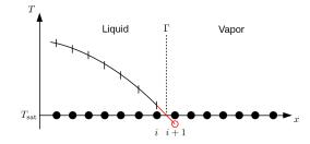
Fig. 4.4 – Representation of a 1D computational domain with liquid on the left of the interface  $\Gamma$ , vapor on the right, and linear extrapolation according to Eq. (4.24) of the liquid temperature field ensuring  $T_{\Gamma} := T_{\text{sat}}$  by the use of the Ghost Fluid Method.
