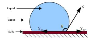
Fig. A.1 – Surfacic energies at contact angle  $\theta$  formed by a liquid droplet lying on a solid surface,  $\gamma_{SL}$  between solid and liquid phases,  $\gamma_{SV}$  between solid and vapor phases and  $\sigma$  between liquid and vapor phases.
