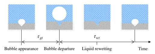
Fig. A.6 – The four steps of the boiling bycle [31].
