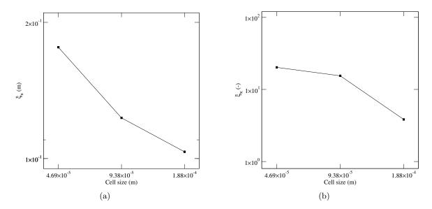
Fig. 6.12 – Error on (a) the final *x*-component of the interface normal vector and relative error on (b) the final interface curvature for the two-dimensional simulations on arbitrary triangles presented in Section 6.6.1.2.
