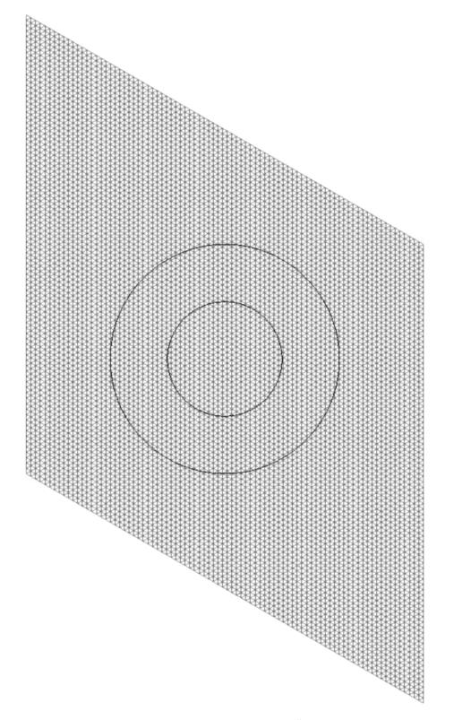
Fig. 6.5 – Coarsest two-dimensional grid ( $\Delta = 9.375 \times 10^{-5} \,\mathrm{m}$ ) composed only of equilateral triangles used is our simulations. The small circle represents the initial interface of radius  $R_0 = 1 \times 10^{-3} \,\mathrm{m}$ , whereas the bigger circle represents the final theoretical interface (the radius is twice the initial one).
