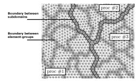
(a) Each core has knowledge of only one subdomain. Each subdomain is divided into element groups to fill the core-specific L1, L2 or L3 caches (see Section 3.1.3.1).
