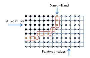
Fig. D.2 – Illustration of the domain partition used in the Fast Marching Method.
