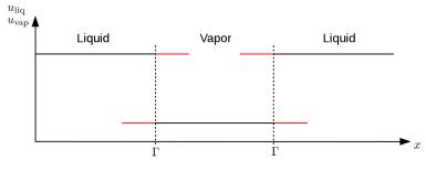
Fig. 4.3 – Constant extrapolations (in red) of the liquid velocity  $\mathbf{u}_{liq}$  in the vapor phase, and of the vapor velocity  $\mathbf{u}_{vap}$  in the liquid phase.
