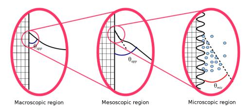
Fig. A.4 – The contact line is described at three different scales : the macroscopic, mesoscopic and microscopic scales. For each scale, a contact angle can be defined [70].
