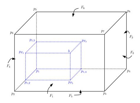
Fig. 3.2 – Contribution  $\mathcal{E}_1$  of the hexahedral element E delimited by nodes  $\mathbf{p}_1, \ldots, \mathbf{p}_8$  to the control volume associated to node  $\mathbf{p}_1$ .
