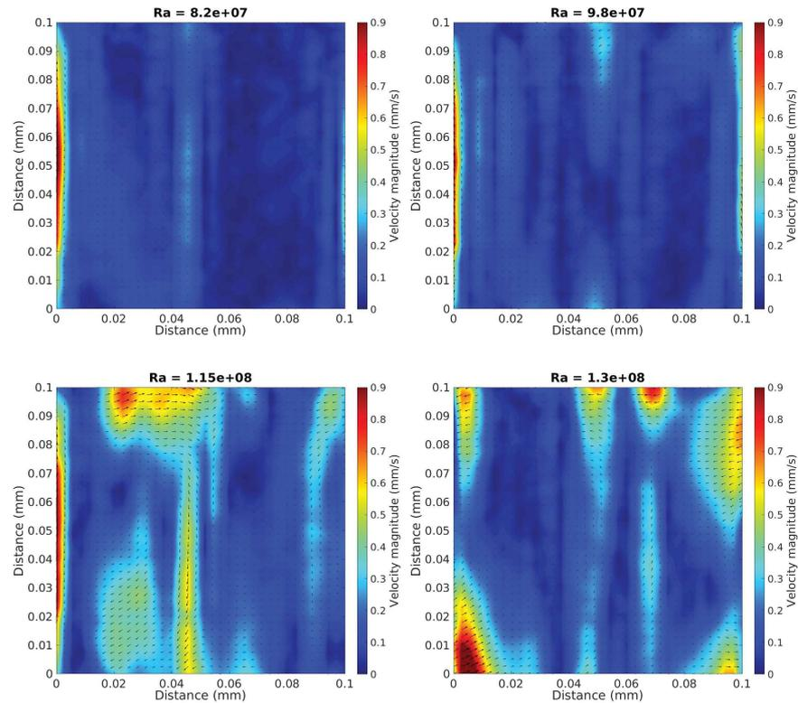
FIGURE 3.29: Mean velocity flow field at a rotation rate of 2.7 rad/s and for  $Ra = 8.2e+07$ ,  $9.84e+07$ ,  $1.15e+08$  and  $1.3e+08$
