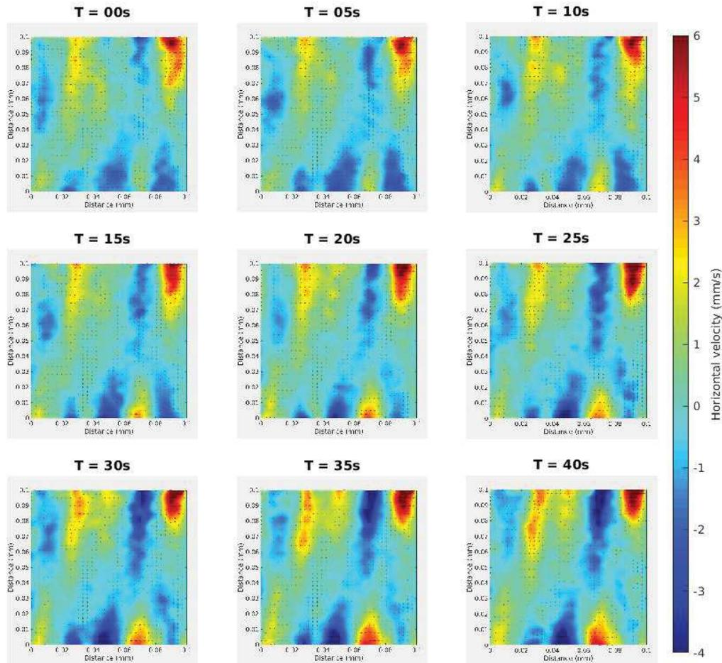
FIGURE 3.6: Instantaneous horizontal velocity at  $Ro = 0.1$ ,  $Ra = 2.7e+08$
