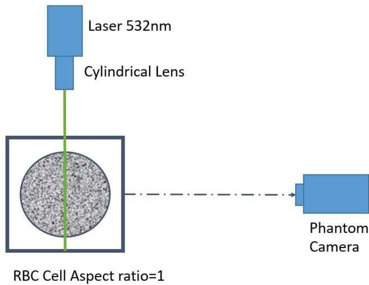
FIGURE 2.13: Particle Image Velocimetry experiment Setup.
