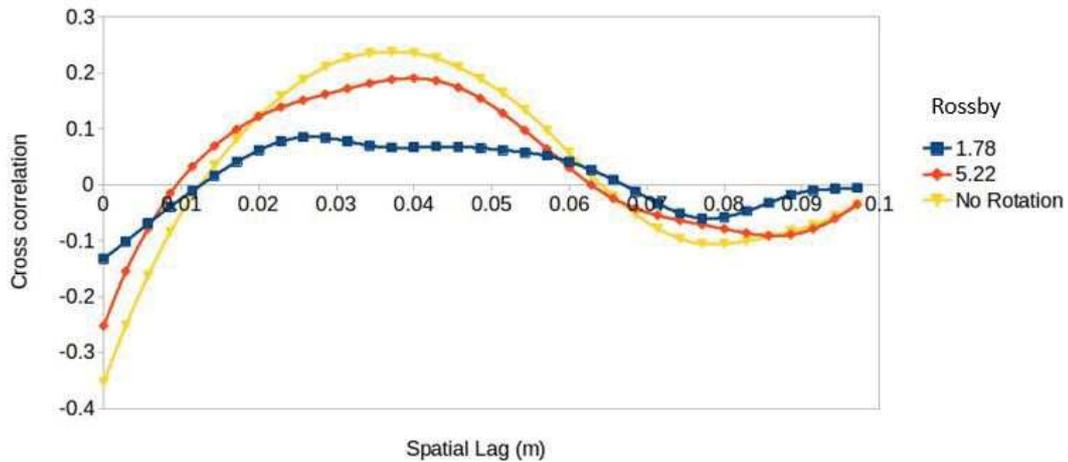
Cross correlation of horizontal component of the velocity near the top and bottom plates ( $Ro < 1$ )
