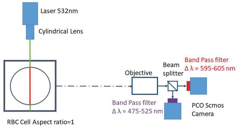
FIGURE 2.8: Laser Induced Fluorescence experimental Setup.
