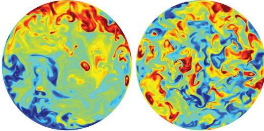
FIGURE 1.12: Temperature field in horizontal mid plane of RBC cell of  $\gamma = 2$ , by Stevens et al., 2010b at  $Pr = 4.38$  and  $Ra = 2.91 \times 10^8$  left  $1/Ro = 0.046$  and right  $1/Ro = 0.6$
