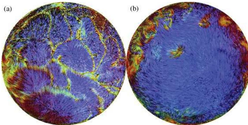
FIGURE 1.5: Thermochromic liquid crystal microsphere image of sheet plumes 2mm (a) and 2cm (b) from the top plate of RBC cell by Zhou et al., 2010
