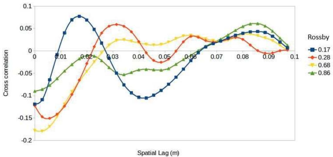
FIGURE 3.13: Cross correlation between the horizontal component of the velocity located near the top and bottom plates for rotation affected regime  $Ro < 1$  (bottom) and rotation unaffected regime  $Ro > 1$  (top).
