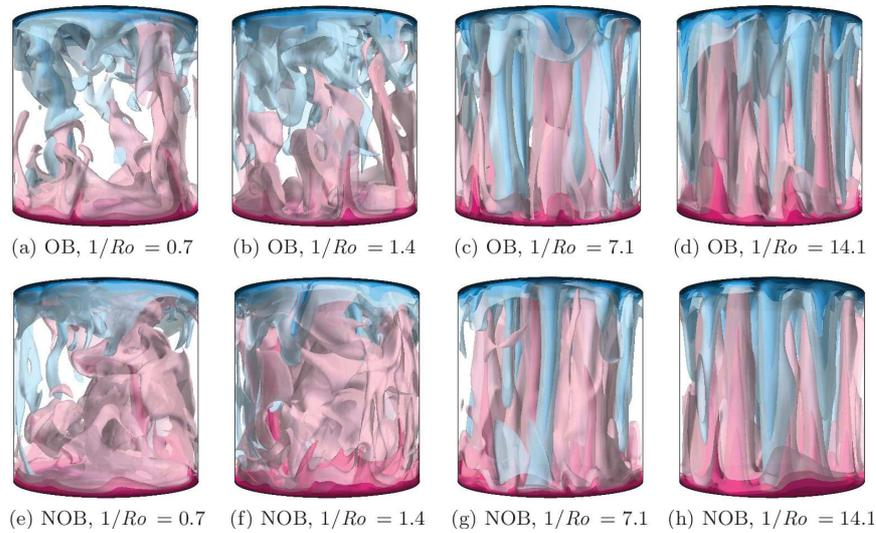
FIGURE 1.6: Instantaneous temperature fields at  $Ra = 10^8$  and  $\Delta T = 40\text{C}$  for NOB studies. Pink represents temperature above mean temperature and blue represents temperature below mean temperature. Horn et al., 2014
