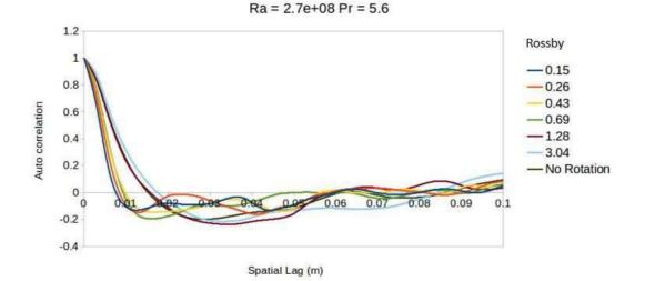
FIGURE 3.21: Auto correlation of vertical component of the velocity near the top plate at Ra = 5.3e+08 (top) and 2.7e+08 (bottom) for different Rossby numbers
