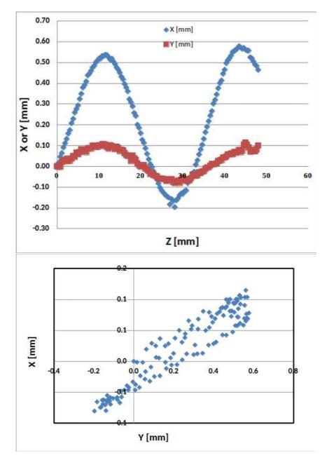
FIGURE 5.7: Planar Zigzag path of bubble in side view of XZ,YZ plane (top) and top view of XY plane (bottom)
