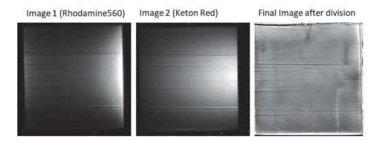
FIGURE 2.11: Images division removes illumination defects
