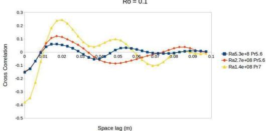
Cross correlation of horizontal component of the velocity near the top and bottom plates Ro = 0.1
