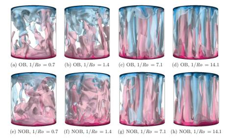
FIGURE 1.6: Instantaneous temperature fields at  $Ra = 10^8$  and  $\Delta T = 40C$  for NOB studies. Pink represents temperature above mean temperature and blue represents temperature below mean temperature. Horn et al., 2014
