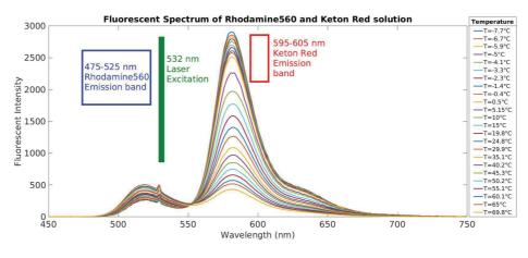
FIGURE 2.2: FLuorescent Spectrum of Rhodamine560 and Kiton Red.
