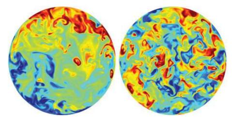
FIGURE 1.12: Temperature field in horizontal mid plane of RBC cell of  $\gamma = 2$ , by Stevens et al., 2010b at Pr = 4.38 and Ra= 2.91 x  $10^8 \text{ left } 1/Ro = 0.046$  and right 1/Ro = 0.6
