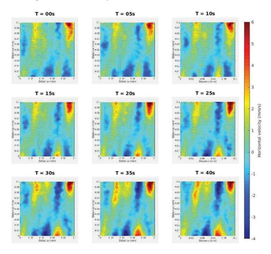
FIGURE 3.6: Instantaneous horizontal velocity at Ro = 0.1 , Ra = 2.7e+08
