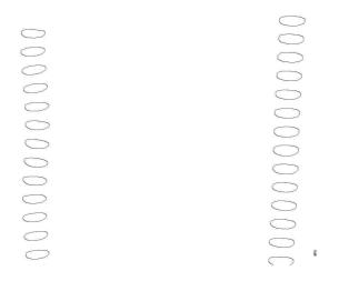
FIGURE 5.6: Bubble planar zigzag trajectory in two orthogonal planes XZ (left) YZ(right) at Bo=6.1 and Ga = 64.6 in silicon oil 10cst.
