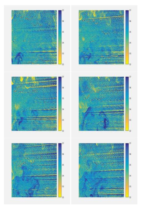
FIGURE 4.1: Instantaneous temperature field without rotation at  $\Delta T = 30^{\circ}C$  and Ra = 8.6e+08. Images are 10s apart.
