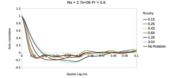
FIGURE 3.20: Auto correlation of vertical component of the velocity near bottom plate at Ra = 5.3e+08 (top) and 2.7e+08 (bottom) for different Rossby numbers
