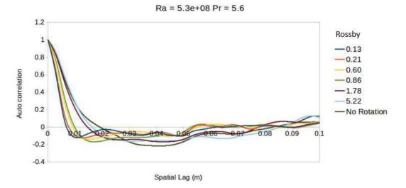
Auto correlation of vertical component of the velocity near bottom plate
