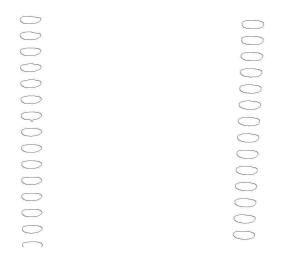
FIGURE 5.5: Bubble rectilinear path in two orthogonal planes XZ (left) YZ(right) at Bo=5.5 and Ga = 60.4 in silicon oil 10cst
