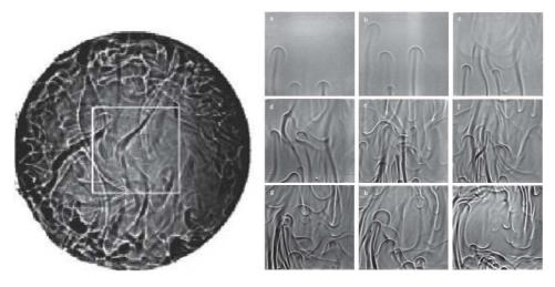
FIGURE 1.4: Shadowgraph technique. Plume visualized from the top view of RBC cell by Funfschilling et al., 2004 (left); Transient large scale flow from front view by Xi et al., 2004 (right).
