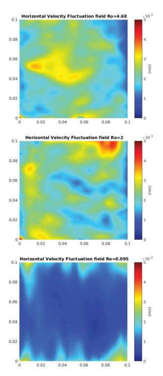
FIGURE 3.24: Horizontal velocity fluctuation at Ro = 4.68 (top), Ro = 2 (middle) and Ro = 0.1 (bottom) for Ra = 2.7e+08..
