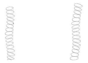
FIGURE 5.8: Bubble helical path in two orthogonal planes XZ (left) YZ(right) at Bo=10 and Ga = 94 in silicon oil 10cst
