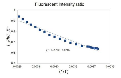
FIGURE 2.6: FLuorescent intensity ratio of Rhodamine560/ Kiton Red in function of the temperature.
