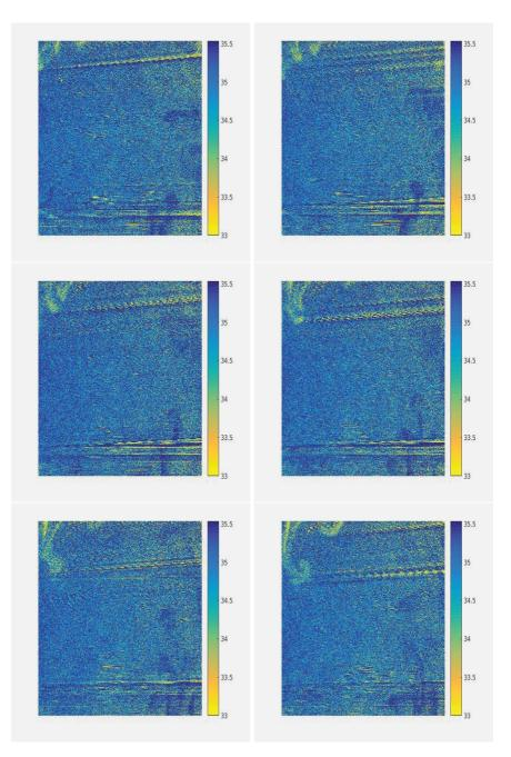
FIGURE 4.2: Instantaneous temperature field without rotation at  $\Delta T = 10^{\circ}C$  and Ra = 2.7e+08. Images are 10s apart.
