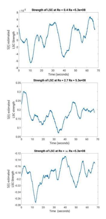
FIGURE 3.5: Temporal evolution of the estimated strength of LSC in the plane of observation at Ro =  $\infty$  (bottom), Ro = 2.7 (middle) Ro = 0.4 (top ).
