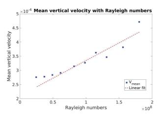
FIGURE 3.30: Mean vertical velocity at various Rayleigh numbers and at a rotation rate of 2.7 rad/s
