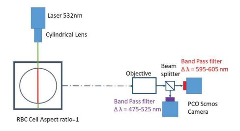
FIGURE 2.8: Laser Induced Fluorescence experimental Setup.
