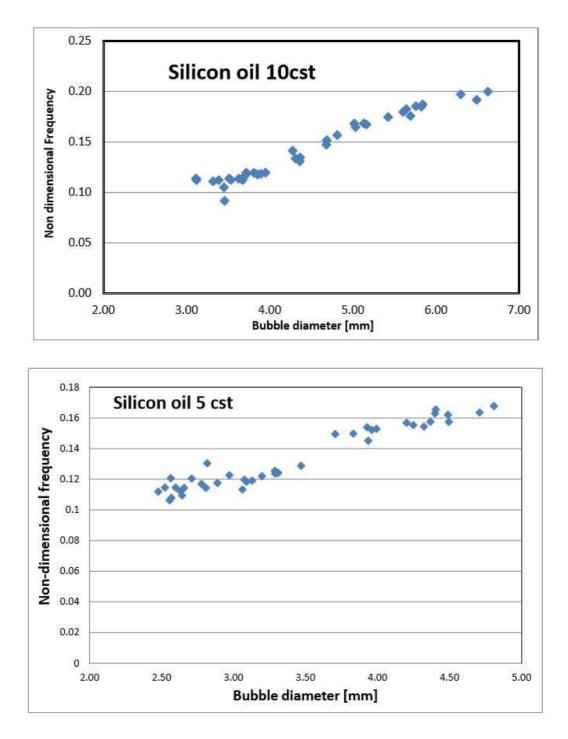
FIGURE 5.11: Non dimensional frequency of oscillation of the rising bubble in silicon oil of 10cst and 5cst.
