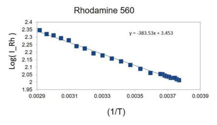
FIGURE 2.4: Fluorescent intensity of Rhodamine560 in function of the temperature.
