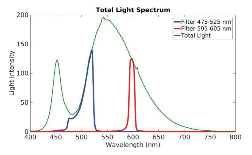
FIGURE 2.3: Fluorescent Emission Spectrum.
