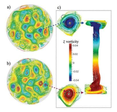
FIGURE 3.2: (a,b) Top view of vorticity near the top and bottom boundary layers (c) Oscillatory vertical column Ribeiro et al Ribeiro et al., 2015
