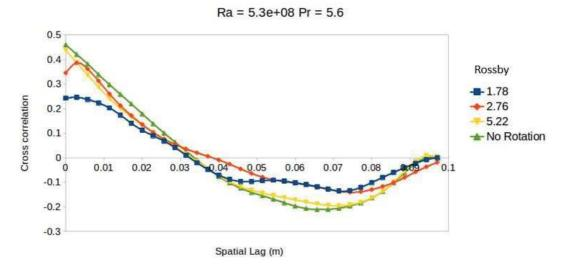
Cross correlation of vertical component of the velocity near the top and bottom plates (Ro > 1)
