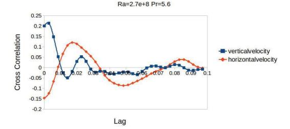
FIGURE 3.19: Horizontal and vertical component of the velocity cross correlation at Ro = 0.1 and Ra = 5.3e+08 (top), 2.7e+08 (bottom)
