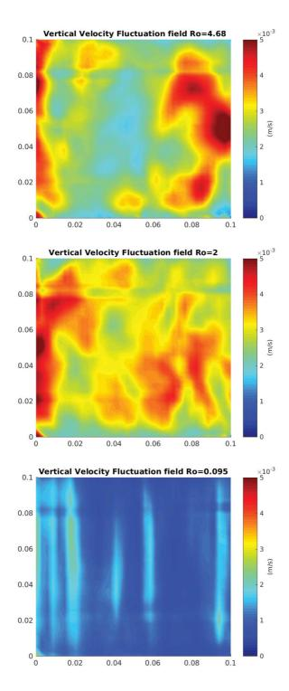
FIGURE 3.23: Vertical velocity fluctuation at Ro = 4.68 (top), Ro = 2 (middle) and Ro = 0.1 (bottom) for Ra = 2.7e+08.
