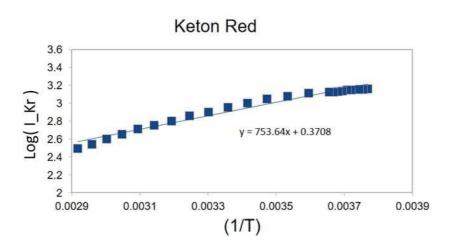
FIGURE 2.5: Fluorescent intensity of Kiton Red in function of the temperature.
