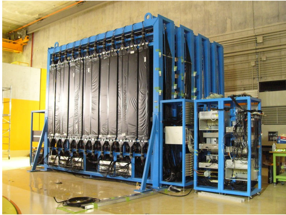
Figure 2.9: Photo of the NEBULA detector in the SAMURAI experimental room at RIKEN.
