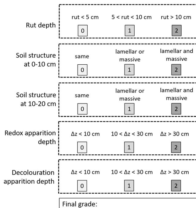
FIGURE 4.1 – Field soil disturbance classification grid
