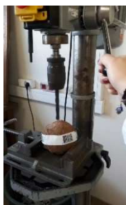
Figure 32. Opening coconut with drilling machine
