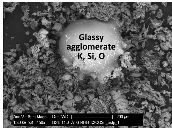
Figure III.27 | SEM observation of ashes from pyrolysis and gasification of rice husks with K 2 CO 3 without contact (same aspect mixed).
