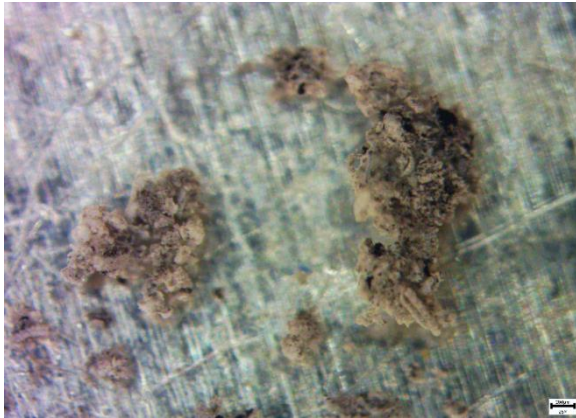
Figure III.23 | Ashes from pyrolysis and gasification of rice husks.
