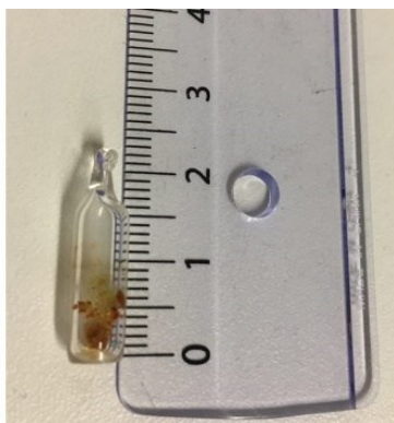
Figure 5.6. Flat bottomed vial to reproduce sealed tube conditions-like during DSC measurements.
