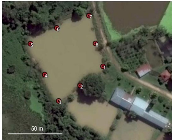
FIGURE 1 Aerial view (Google © DigitalGlobe 2016) of the zone where the experimental pond ( 8^{\circ}24'02''S – 74^{\circ}38'26''W ) is situated and positions of the eight hydrophones (numbered circles) forming the array inside the pond
